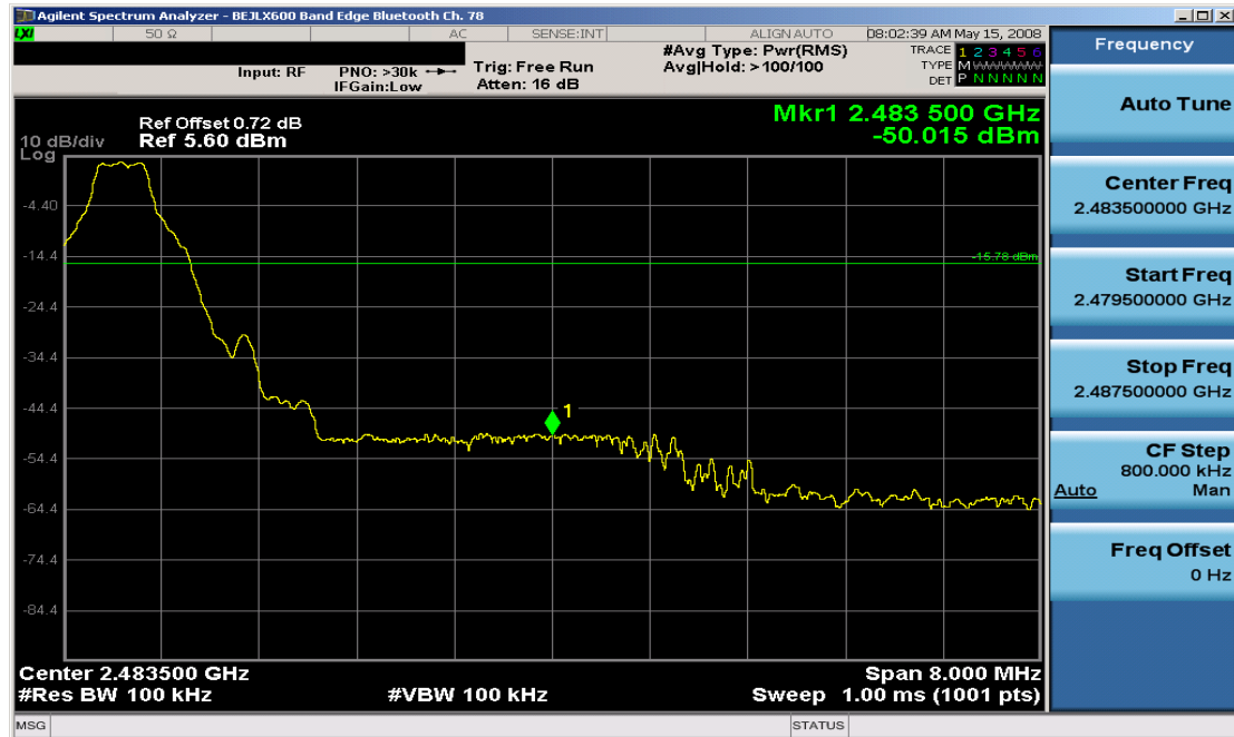
Plot 6-5. Band Edge Plot (Bluetooth – Ch. 78)
