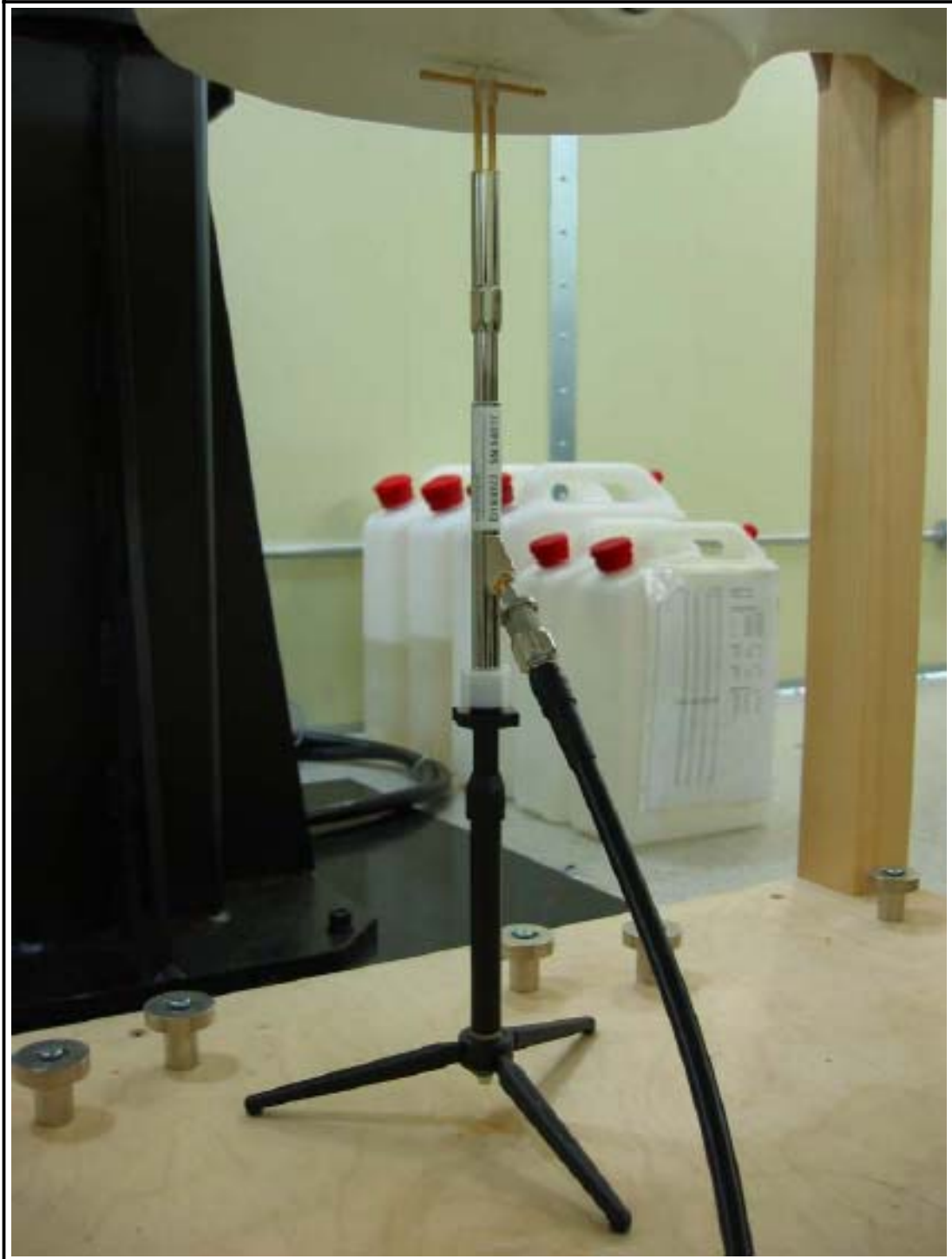
Figure 2 1900 MHz Dipole Validation Test Setup
