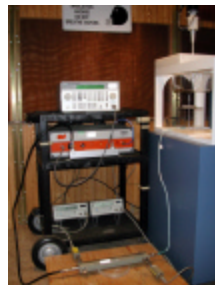
Figure A.0 Dipole Validation Test Setup
