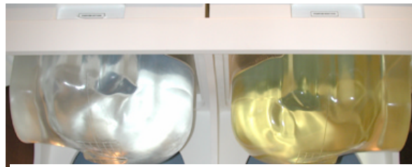
Figure 7.1 Left and Right SAM Phantom shells
