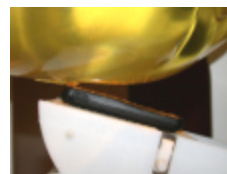
Figure A.6 Right Head SAR Test Setup -- Ear / 15° Tilt Position --
