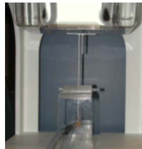
Figure A.0 Dipole Validation Test Setup
