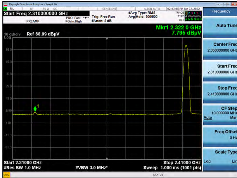
Radiated Restricted Band Edges plot – Peak Result (Ch.0, H)
