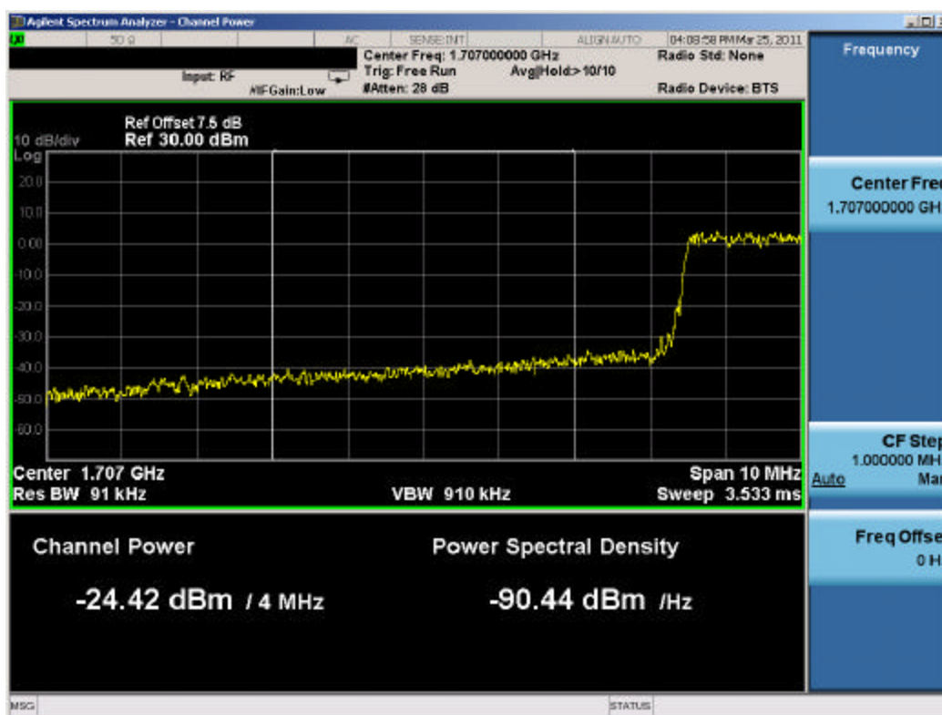
Plot 7-46. Extended Band Edge Plot (10MHz BW, QPSK, AWS Band – Low Channel)
