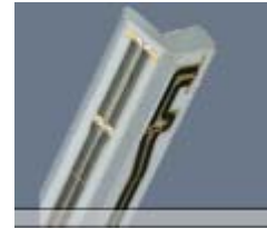
Figure 5-1 E-field Free-space Probe
