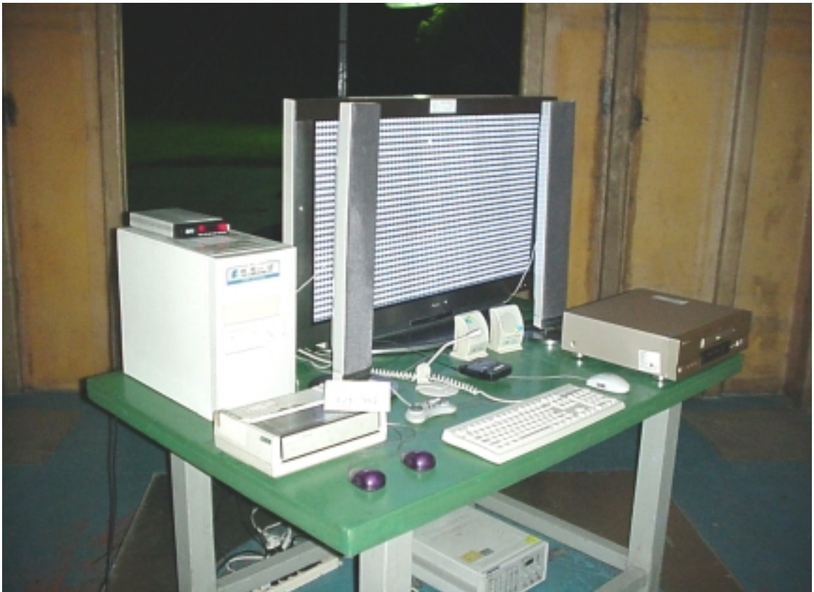
SETUP WITH MAXIMUM DETECTED EMISSION AT VERTICAL POLARIZATION
