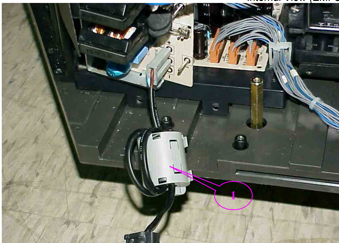
Figure 10 Internal View (EMI Core)
