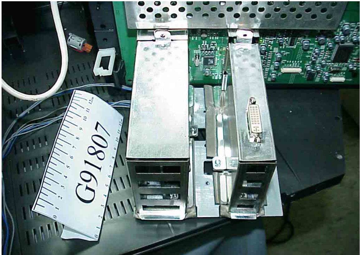
Figure 31 Internal View (I/O Control Board)
