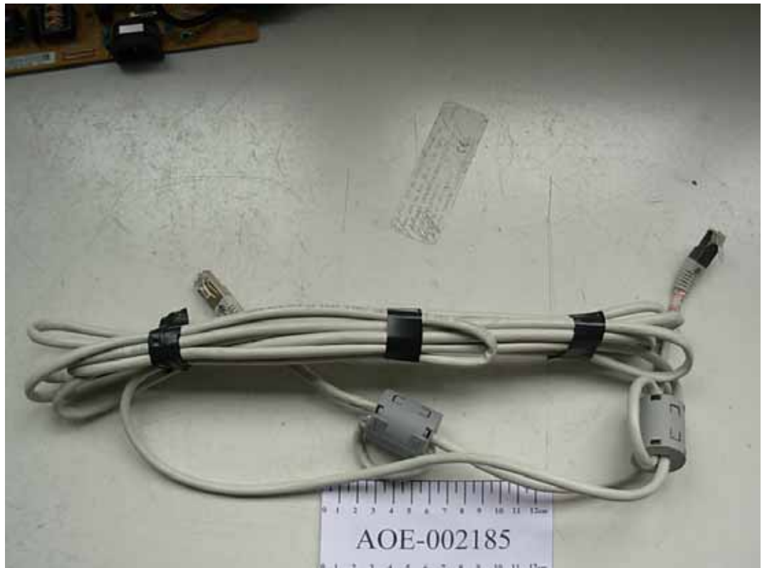
FIGURE 7 NETWORK MONITOR (M/N: N1642WT) STP CABLE
