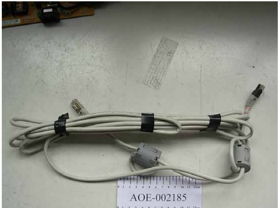
FIGURE 7 NETWORK MONITOR (M/N: N1742LET) STP CABLE
