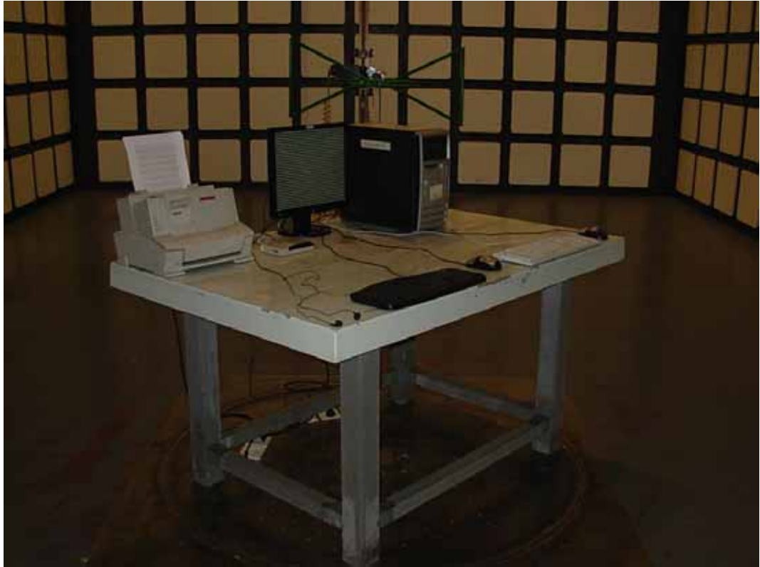
SETUP WITH MAXIMUM DETECTED EMISSION AT HORIZONTAL POLARIZATION (X-PORT 800*600@72Hz)
