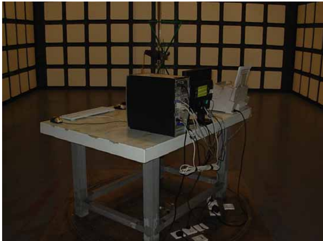
SETUP WITH MAXIMUM DETECTED EMISSION AT VERTICAL POLARIZATION (X-PORT 800*600@72Hz)
