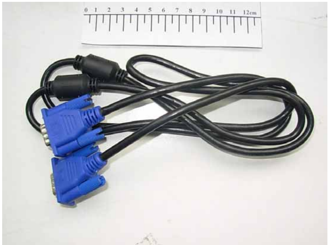
FIGURE 6 NETWORK MONITOR (M/N: N1941WT) D-SUB CABLE #1
