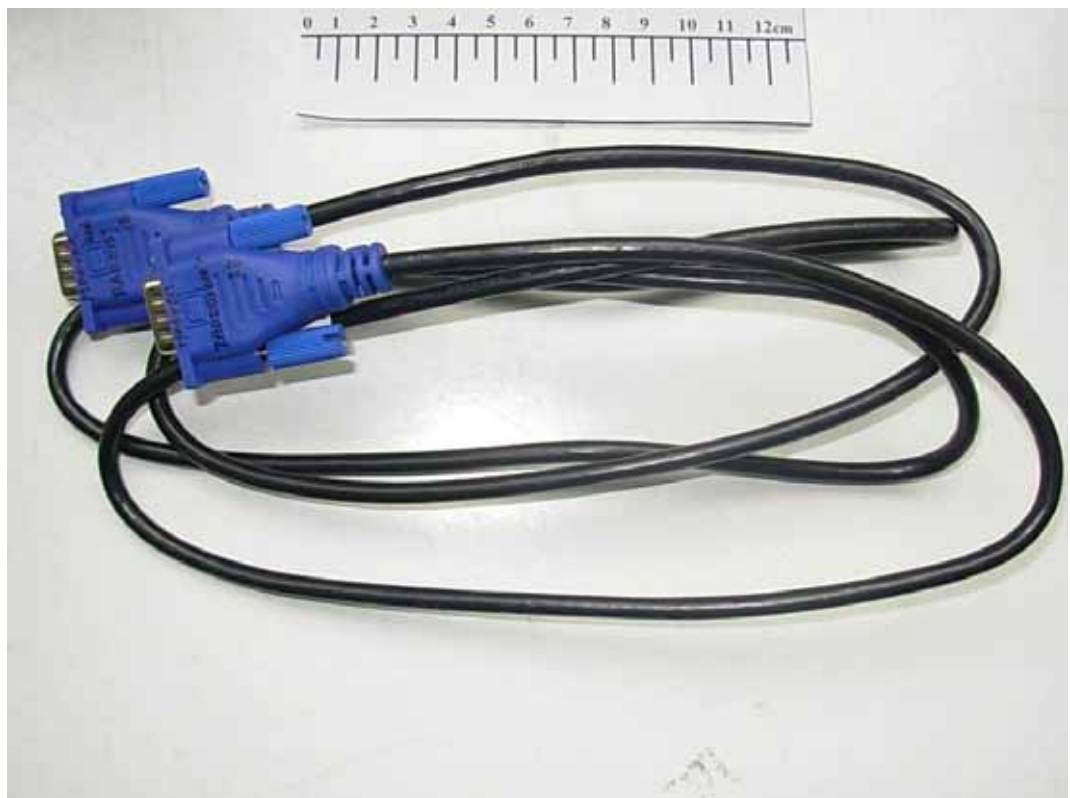
FIGURE 7 NETWORK MONITOR (M/N: N1941WT) D-SUB CABLE #2
