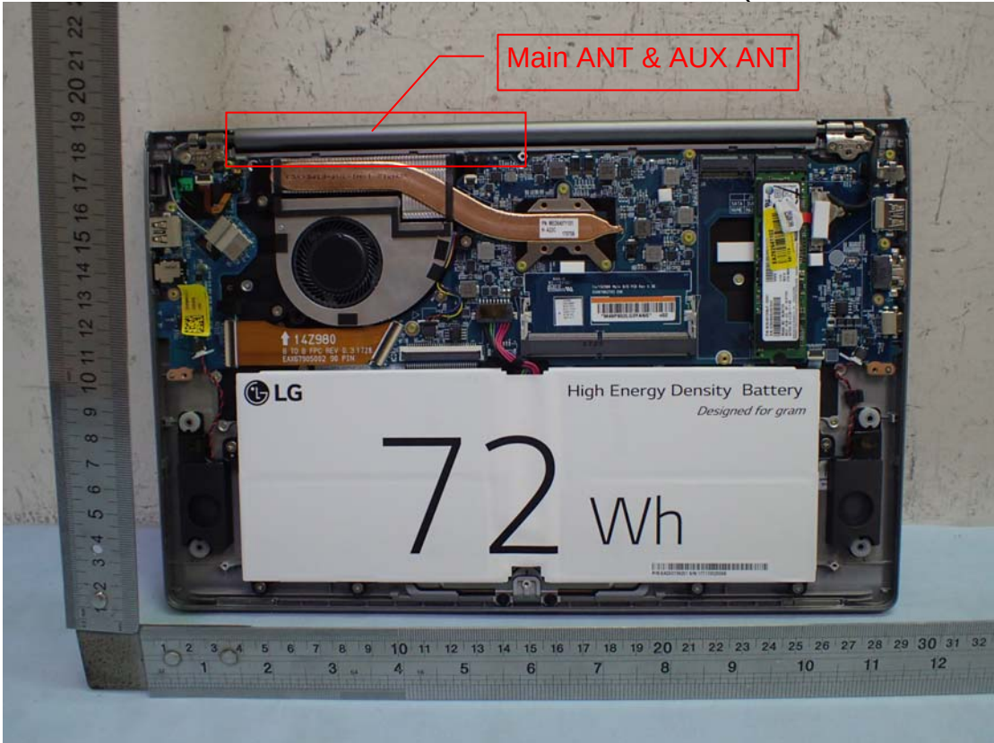
Figure 26 Internal View (Antenna & Position)
