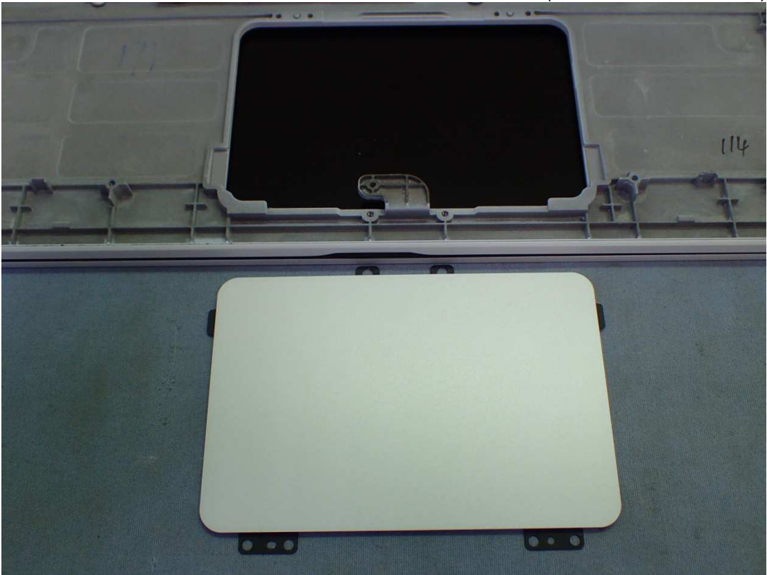
Figure 18 Internal View (Removed Touch Pad)
