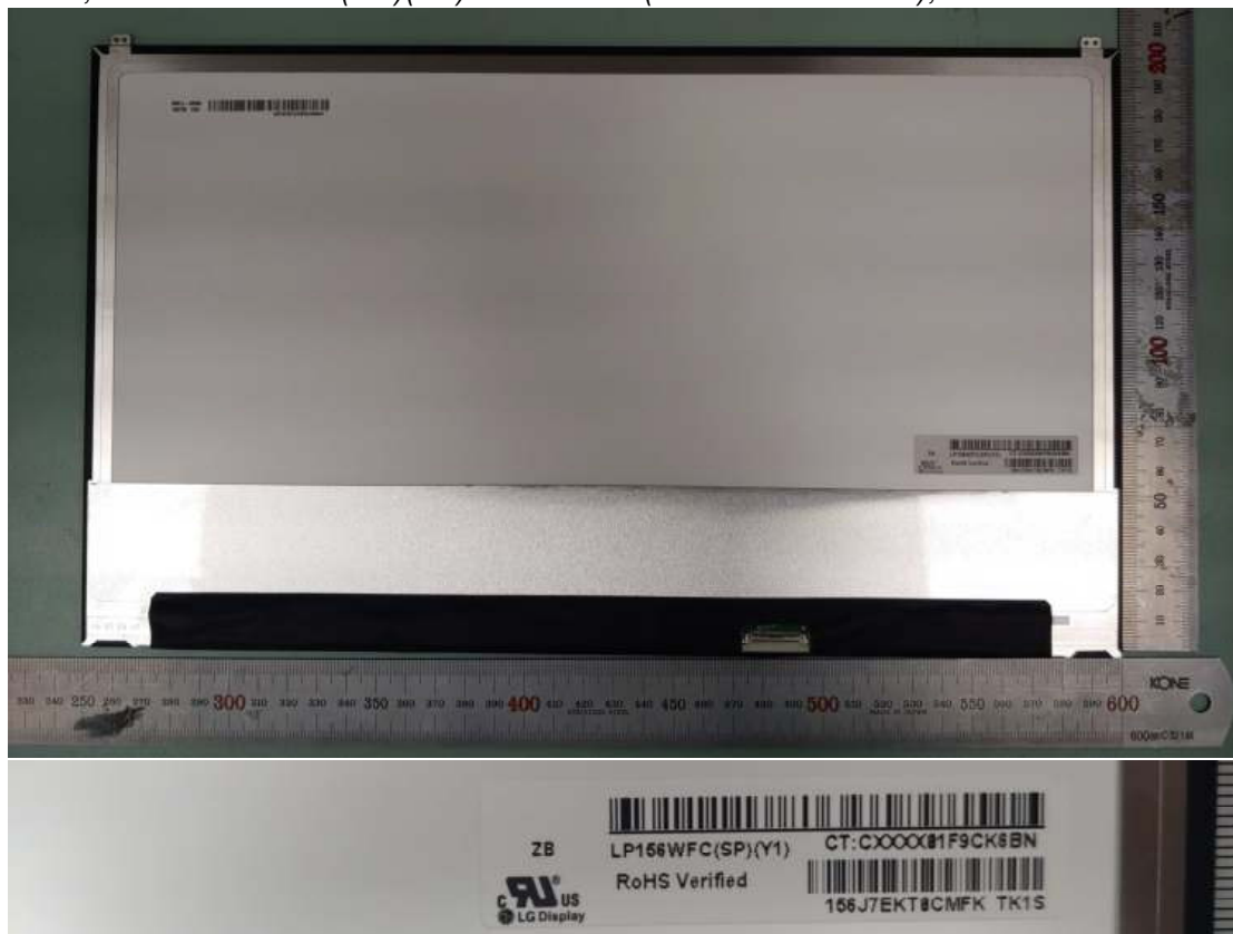
Figure 34 LGD, M/N LP156WFC(SP)(Y1) LCD Panel (Normal Non touch), Back View/ Label View
