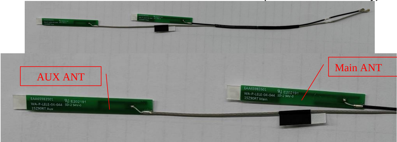
Figure 20 WLAN Combo Antenna (Main Black / AUX Gray)
