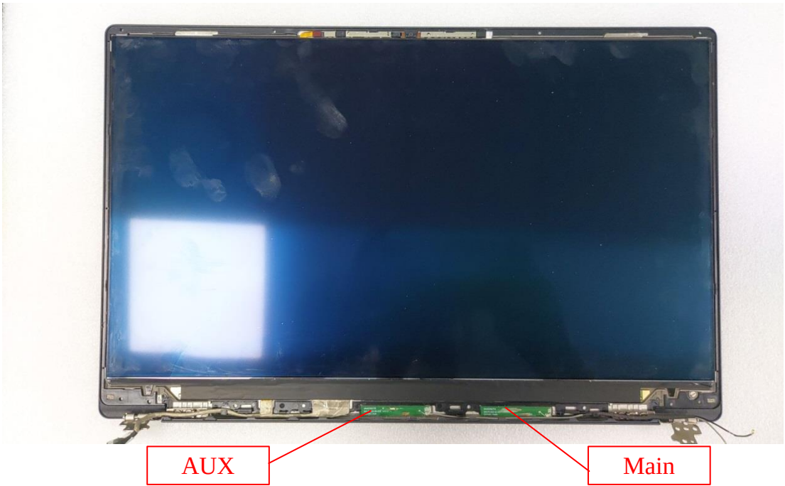
Figure 20 WLAN Combo Antenna (Main Black / AUX Gray)
