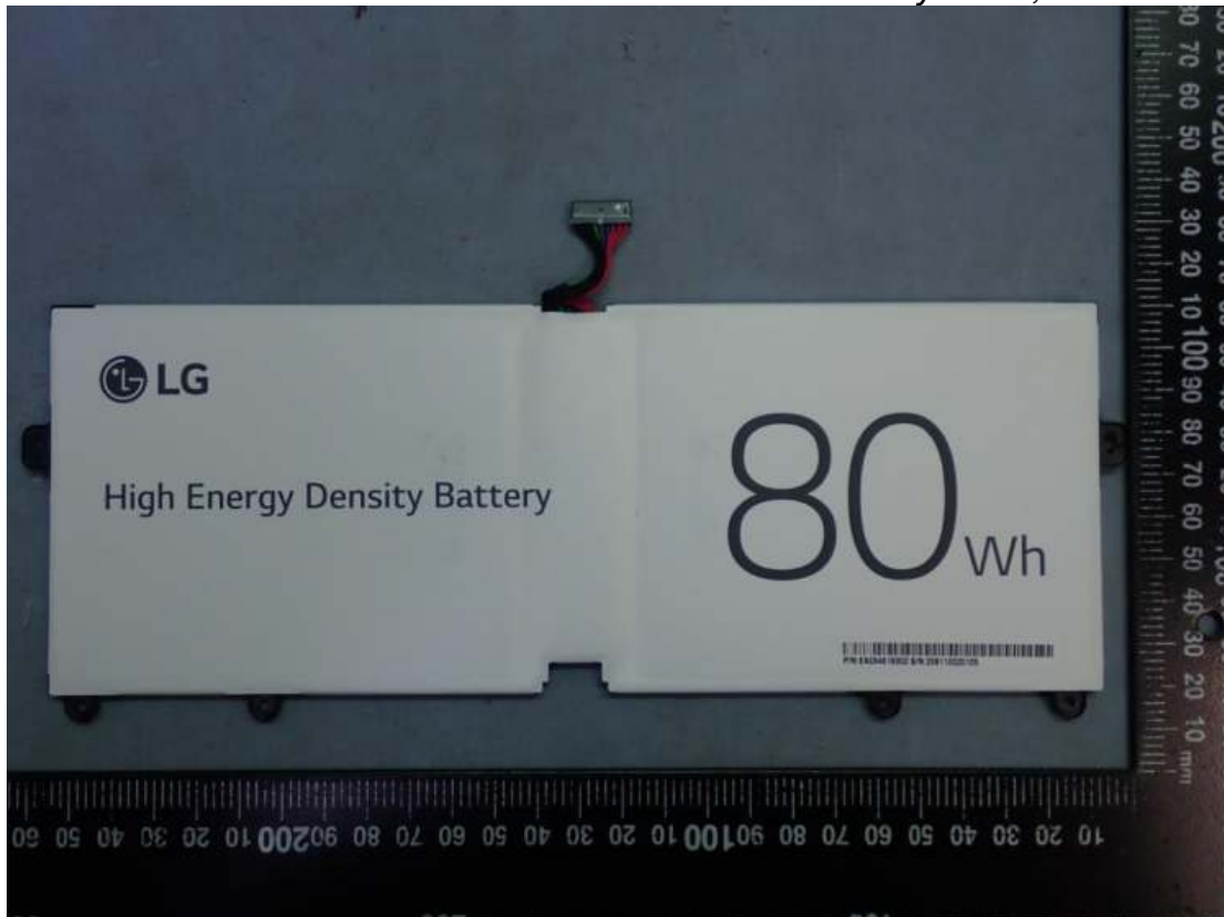
Figure 35 Battery Pack, Front View
