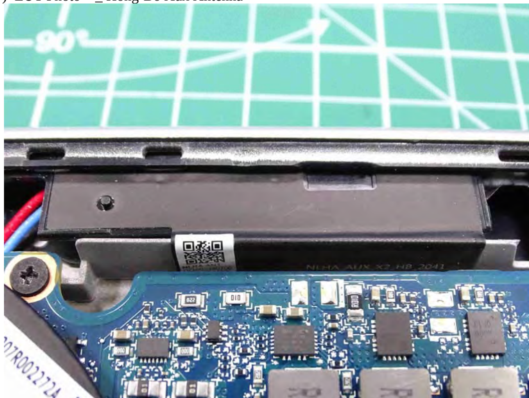
(18) EUT Photo _ Yageo Main Antenna
