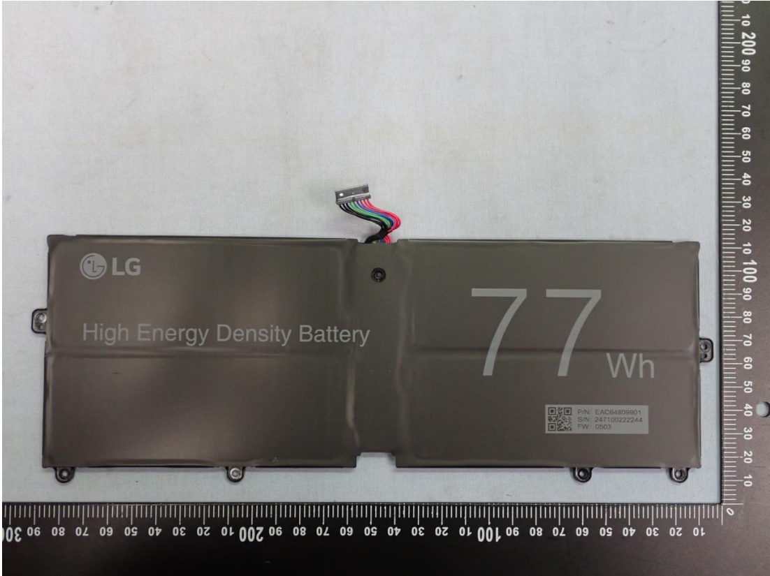
Figure 39 Battery, Front View
