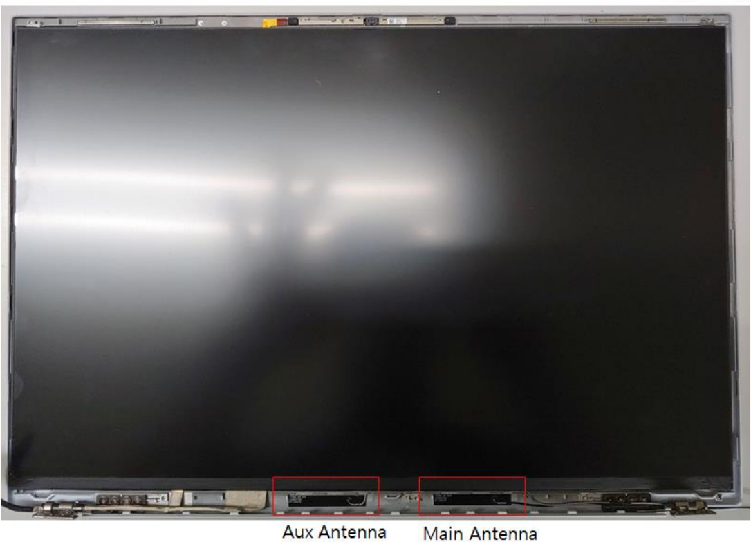
Figure 32 L1LRF009-CS-H, WLAN Combo Antenna Position
