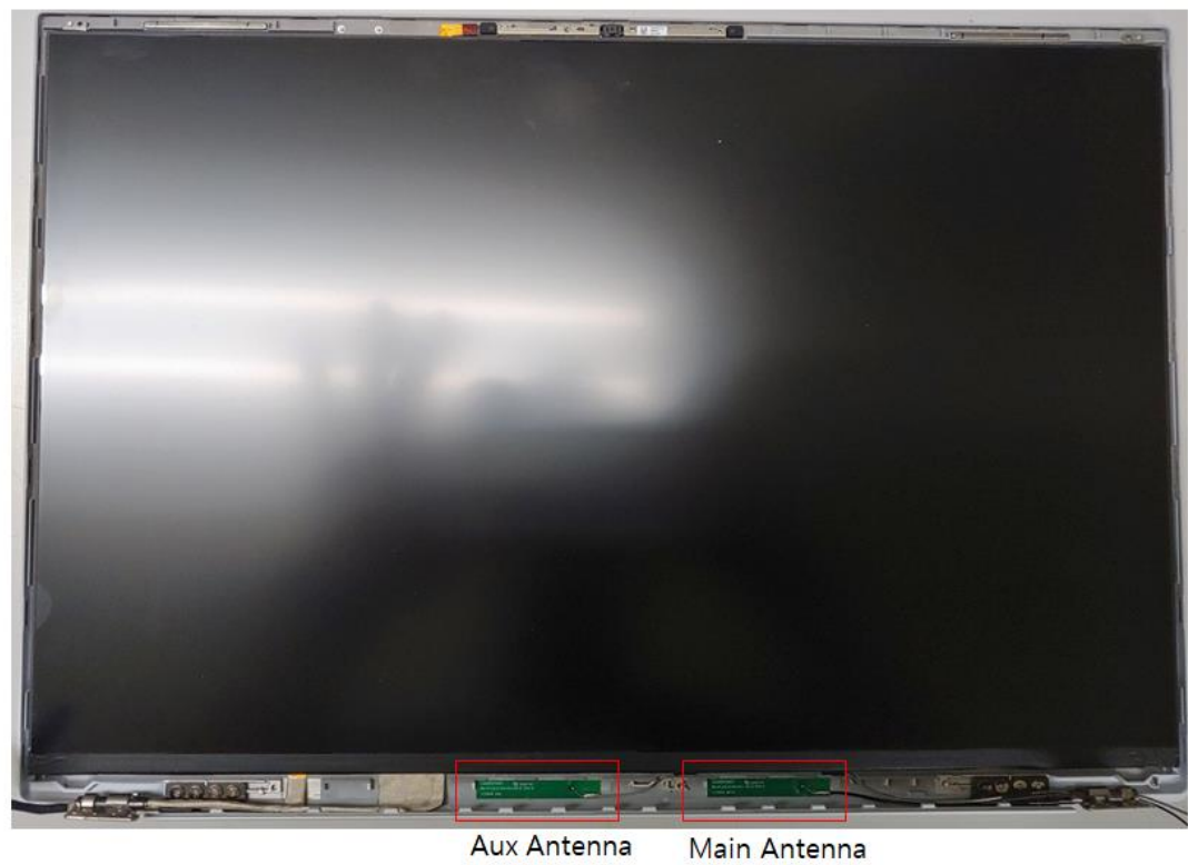
Figure 31 WA-P-LELE-04-011, WLAN Combo Antenna Position
