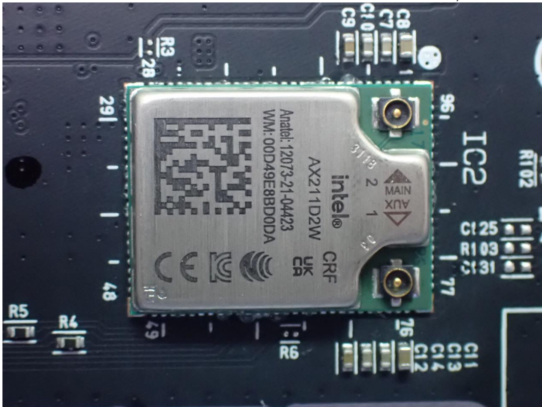
Figure 21 WLAN Combo Card, Front View
