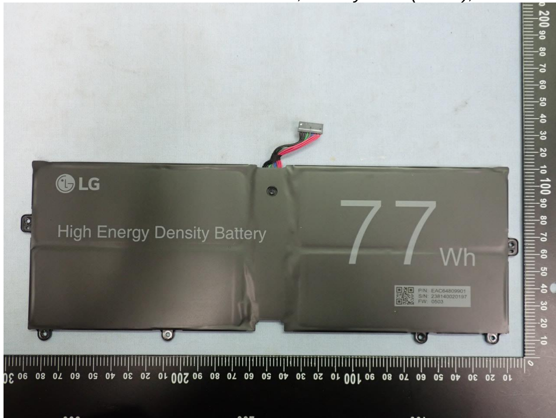
Figure 23 This Time add, Battery Pack (77Wh), Front View
