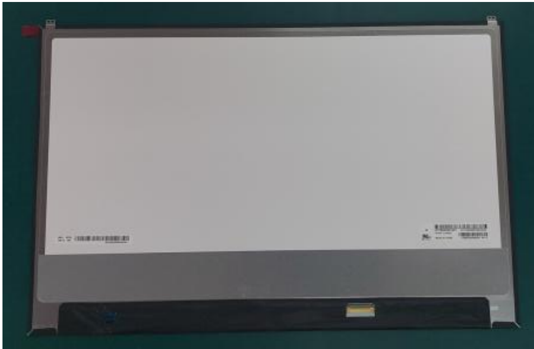
Figure 47 LP170WQ2 (SP)(B1), LCD Panel, Back View/Label View
