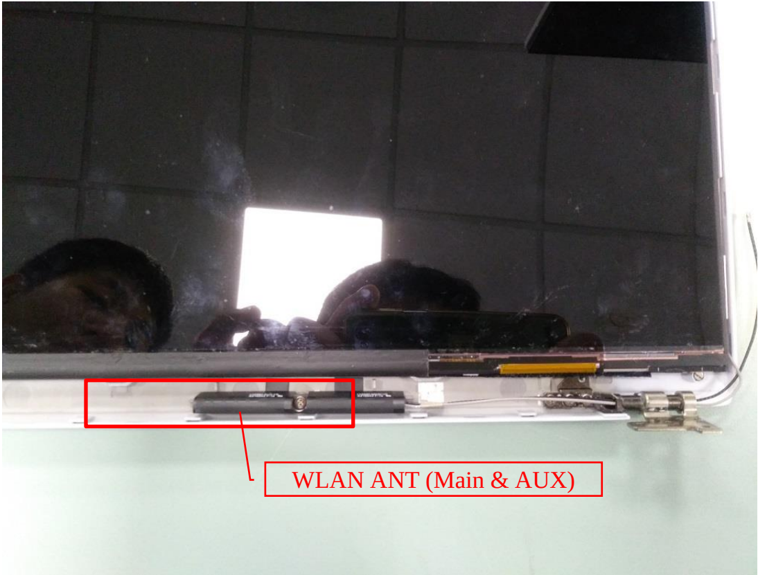
Figure 44 WLAN Antenna Position
