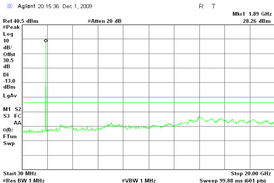
Figure 8-3: Out of Band emission at antenna terminals – GPRS CH High
