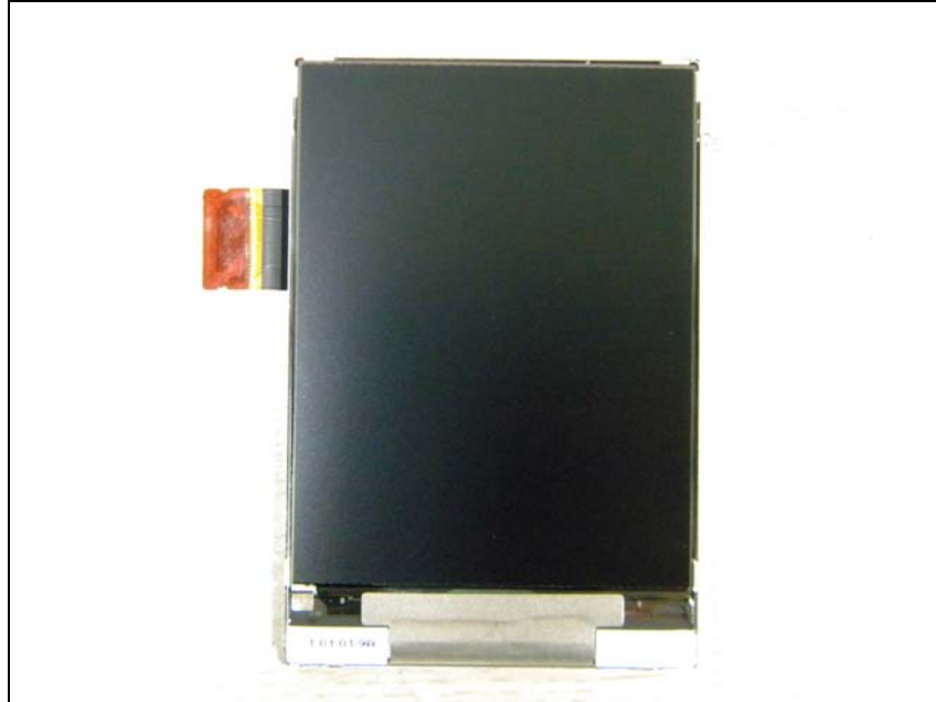
Bottom view of LCD Panel
