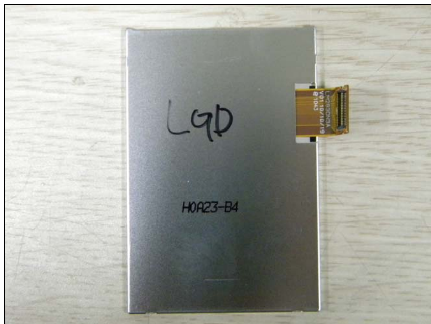
Bottom view of LCD Panel
