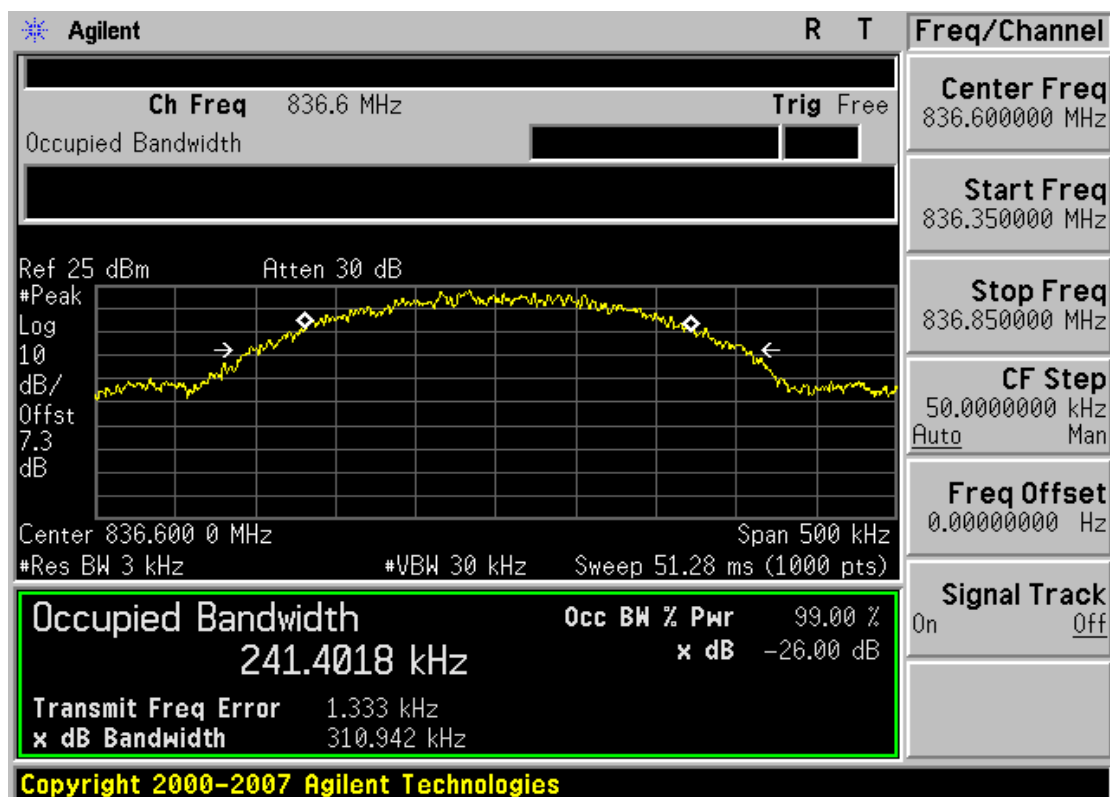
Plot 7-10. Occupied Bandwidth Plot (EDGE850 Mode – Ch. 190)
