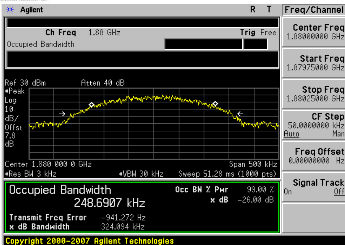
Plot 7-21. Occupied Bandwidth Plot (EDGE1900 Mode – Ch. 661)
