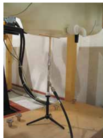
Photo of the dipole Antenna
