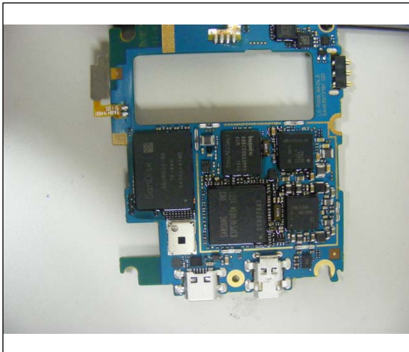
Bottom view of main board
