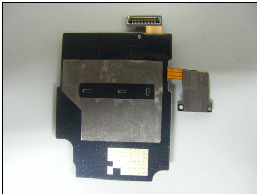
Bottom view of SIM card board
