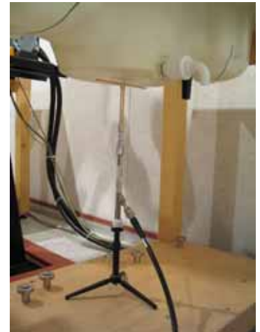
Photo of the dipole Antenna
