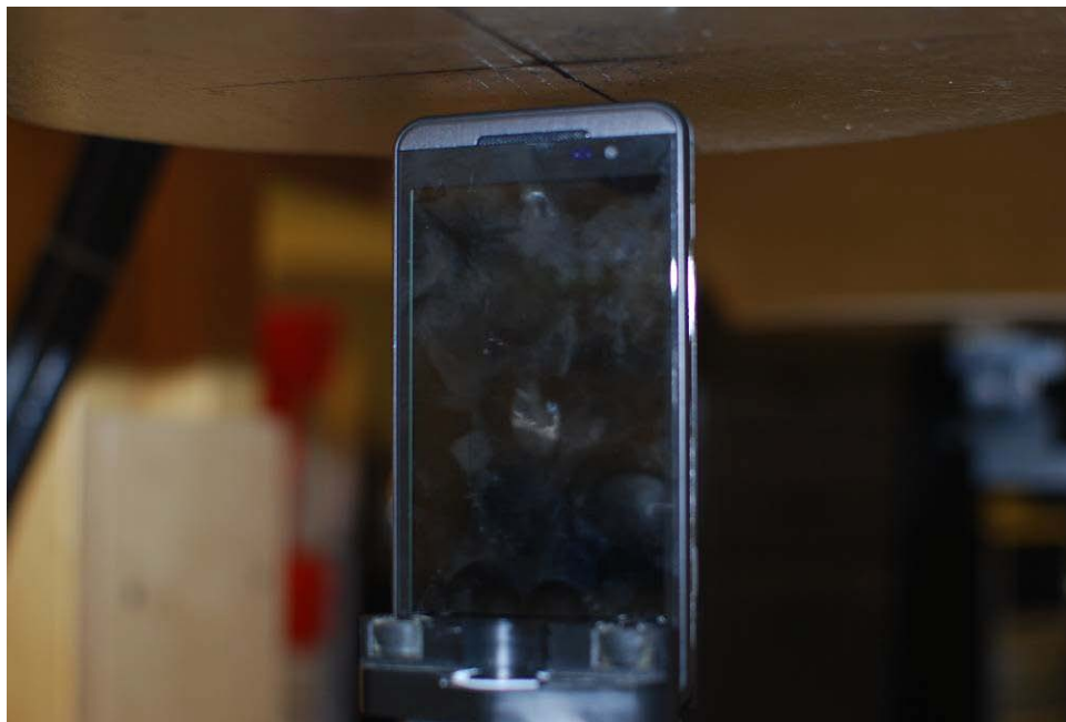
Figure 21-10 SAR Test Setup Photo 10: Top Edge 1.0 cm
