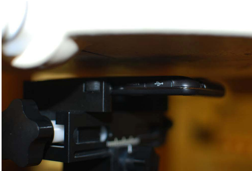
Figure 21-5 SAR Test Setup Photo 5: Back 1.0 cm
