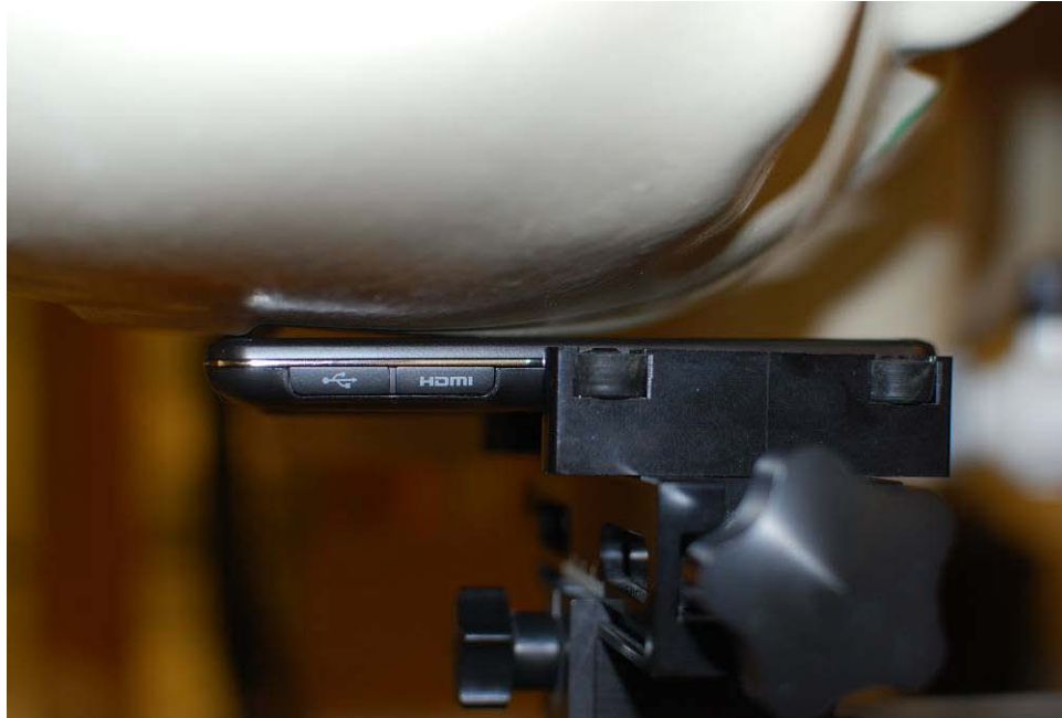
Figure 21-1 SAR Test Setup Photo – Right Touch
