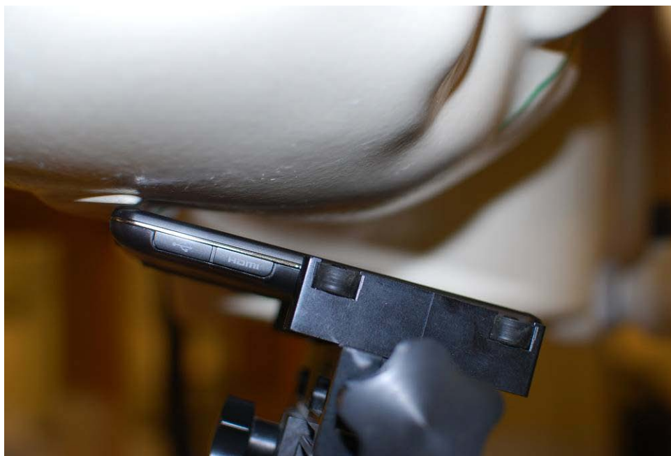
Figure 21-2 SAR Test Setup Photo – Right Tilt
