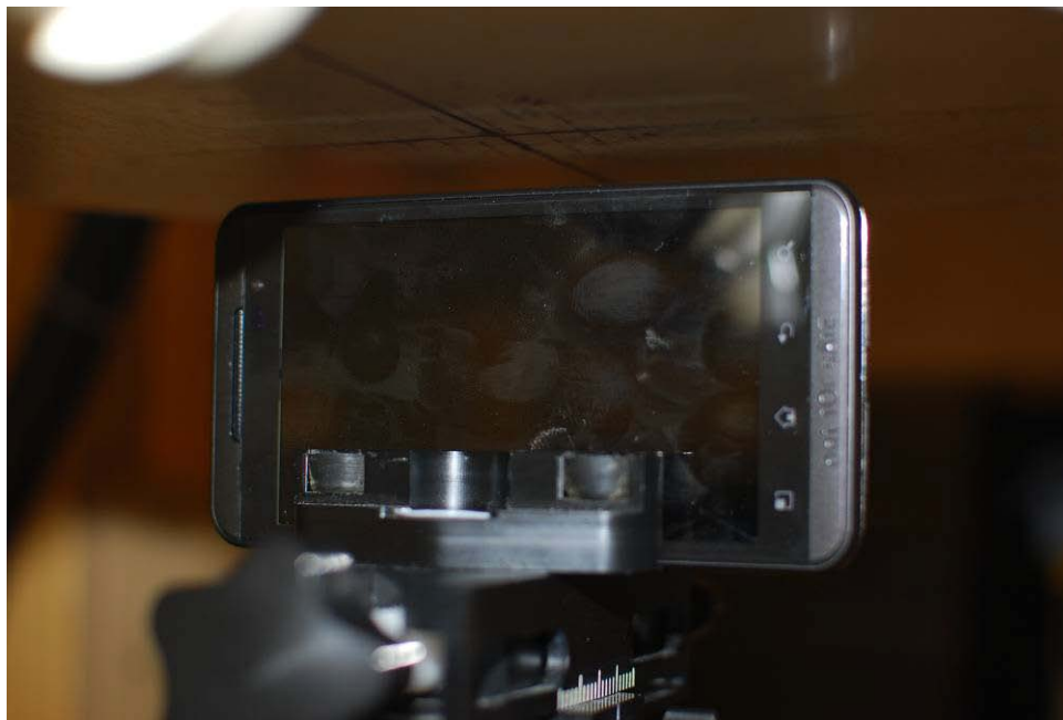
Figure 21-8 SAR Test Setup Photo 8: Right Edge 1.0 cm
