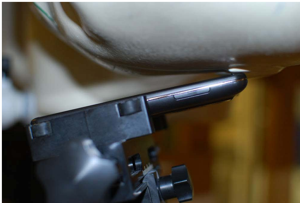
Figure 21-4 SAR Test Setup Photo – Left Tilt
