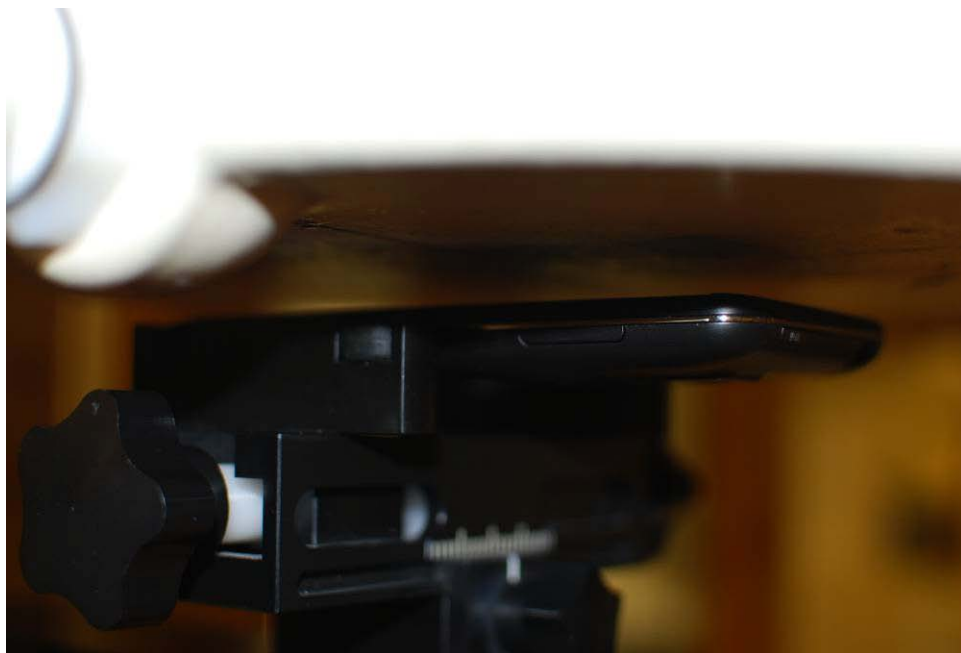
Figure 21-6 SAR Test Setup Photo 6: Front 1.0 cm
