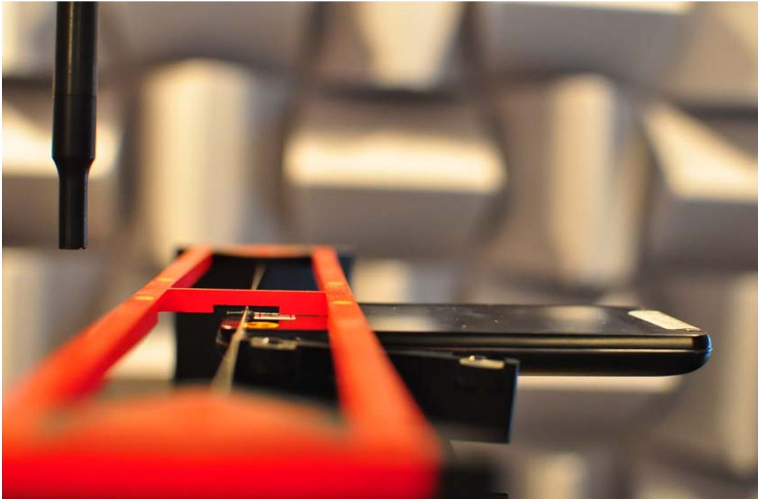
Figure 17-2 HAC Phantom Plane Alignment
