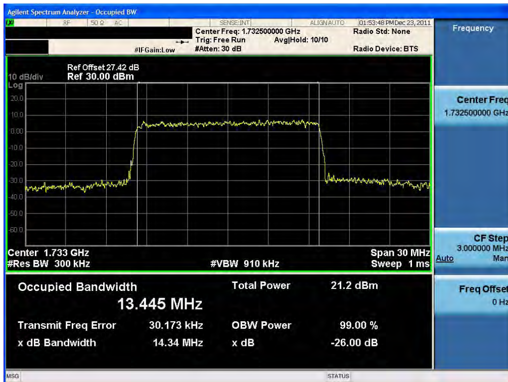
Occupied Bandwidth Plot (15 MHz BW, 16QAM, Band 4 – Mid Channel) RB75-0
