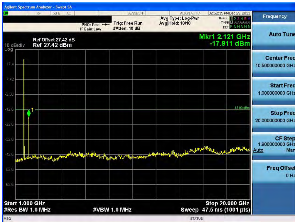
Conducted Spurious Plot (15 MHz BW, QPSK, Band 4 – Mid Channel) RB36–18
