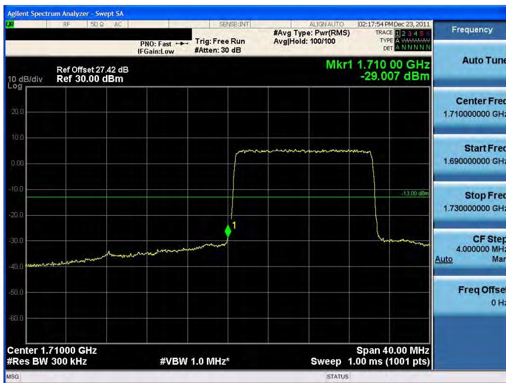
BAND EDGE Plot (15 MHz BW, 16QAM, Band 4 – Low Channel) RB75-0
