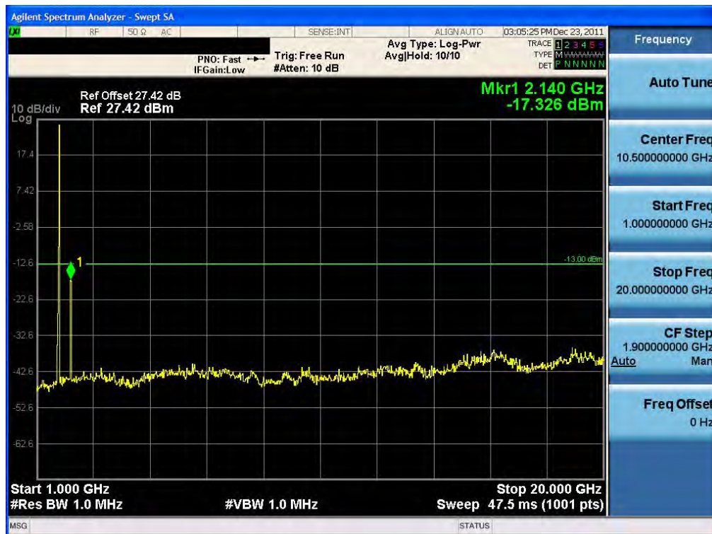
Conducted Spurious Plot (15 MHz BW, 16QAM, Band 4 – High Channel) RB1-74
