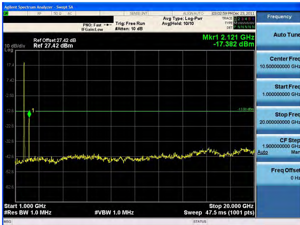
Conducted Spurious Plot (15 MHz BW, QPSK, Band 4 – Low Channel) RB75-0
