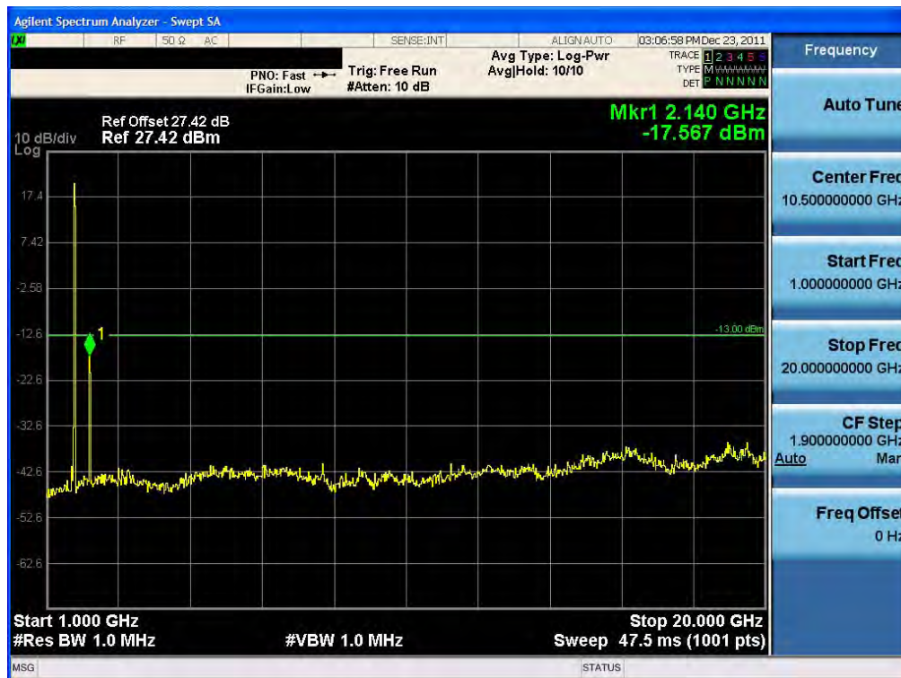
Conducted Spurious Plot (15 MHz BW, 16QAM, Band 4 – High Channel) RB36-18
