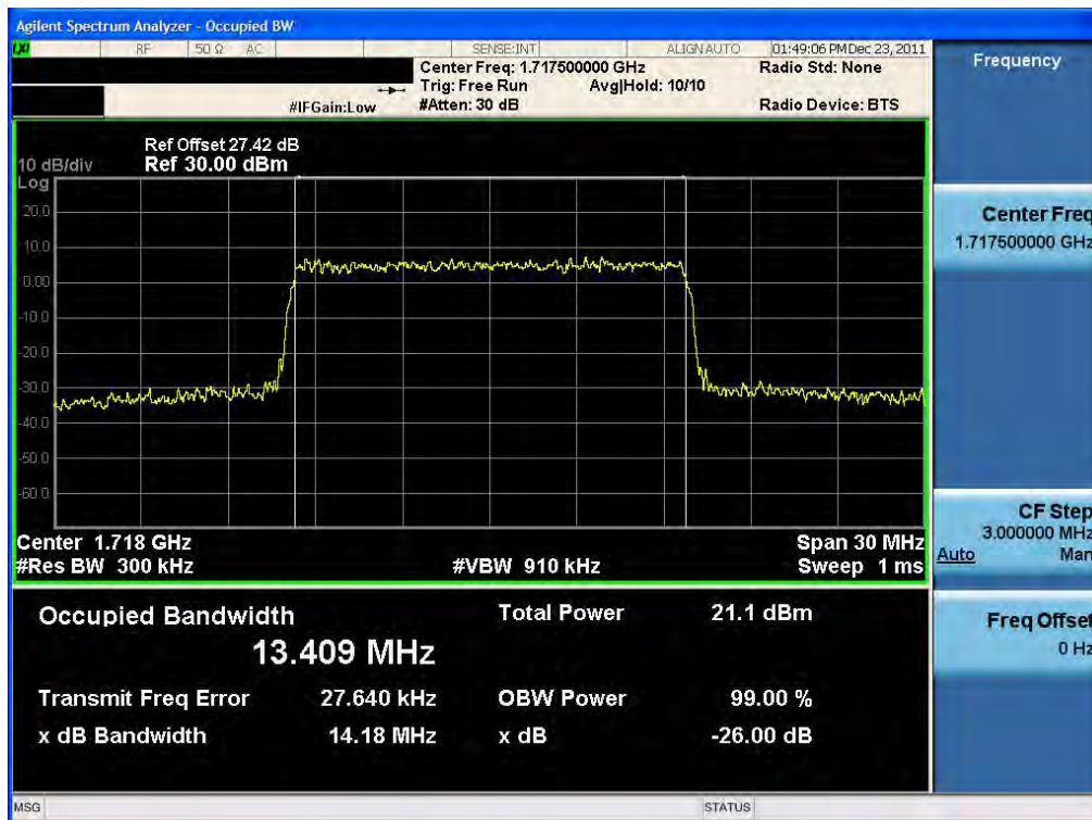
Occupied Bandwidth Plot (15 MHz BW, 16QAM, Band 4 -Low Channel) RB75-0
