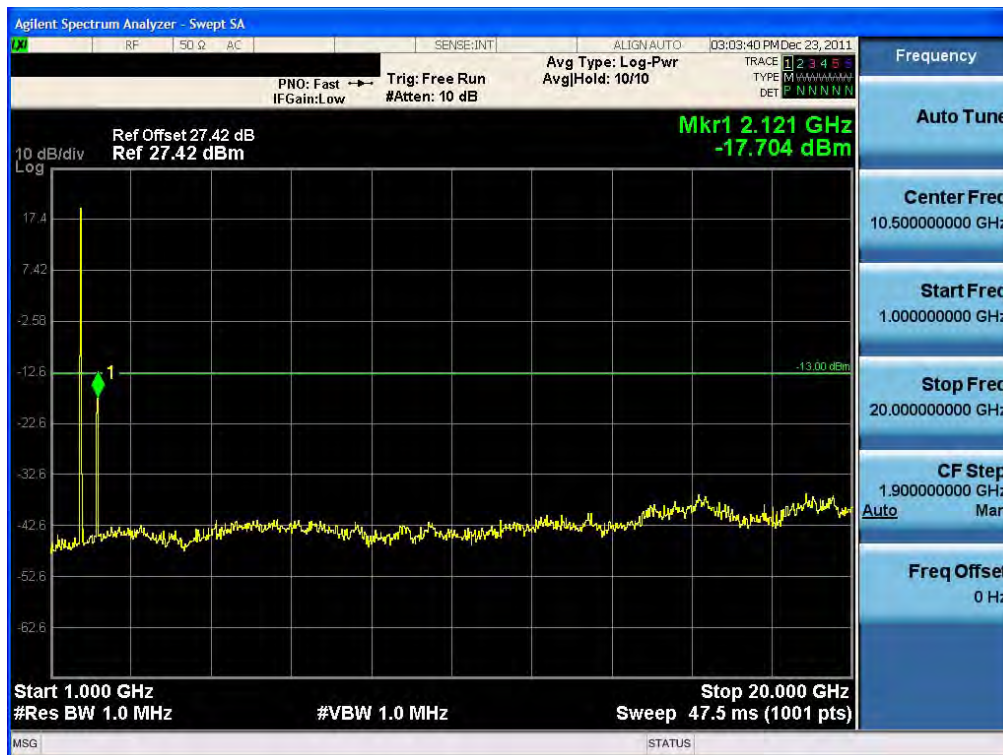
Conducted Spurious Plot (15 MHz BW, 16QAM, Band 4 – Low Channel) RB36–18
