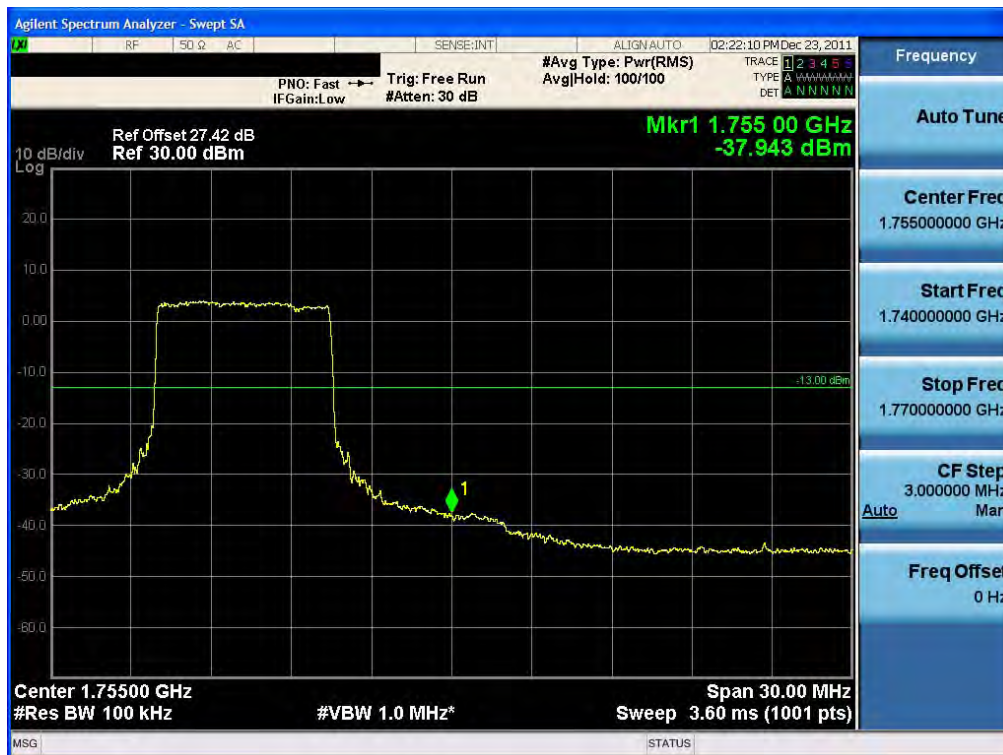
BAND EDGE Plot (15 MHz BW, 16QAM, Band 4 – High Channel) RB36-18
