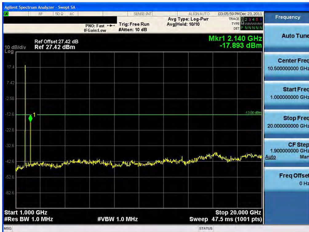
Conducted Spurious Plot (15 MHz BW, 16QAM, Band 4 – High Channel) RB75-0
