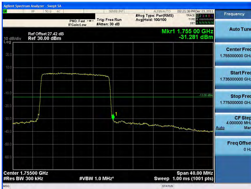
BAND EDGE Plot (15 MHz BW, 16QAM, Band 4 – High Channel) RB75-0
