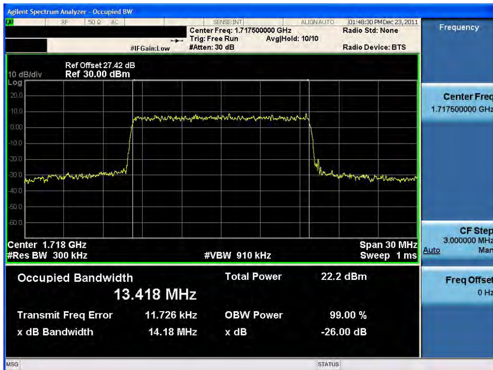
Occupied Bandwidth Plot (15 MHz BW, QPSK, Band 4 -Low Channel) RB75-0
