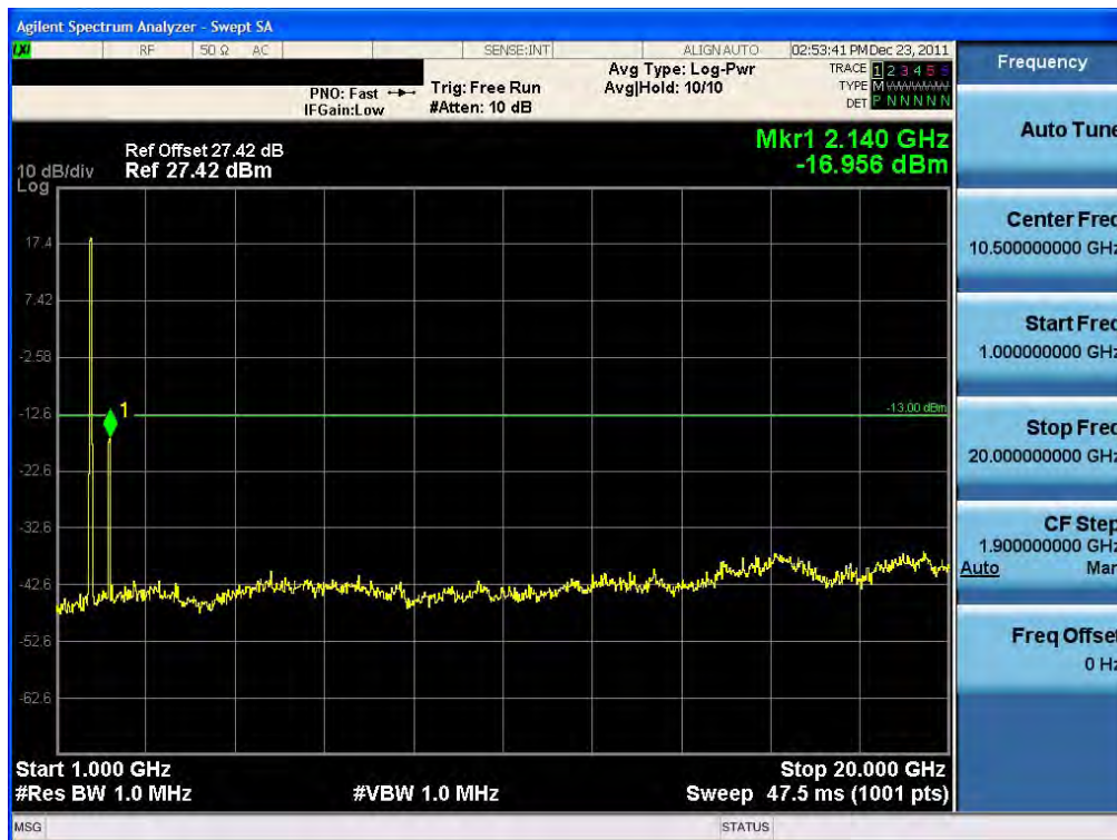
Conducted Spurious Plot (15 MHz BW, QPSK, Band 4 – Mid Channel) RB75-0
