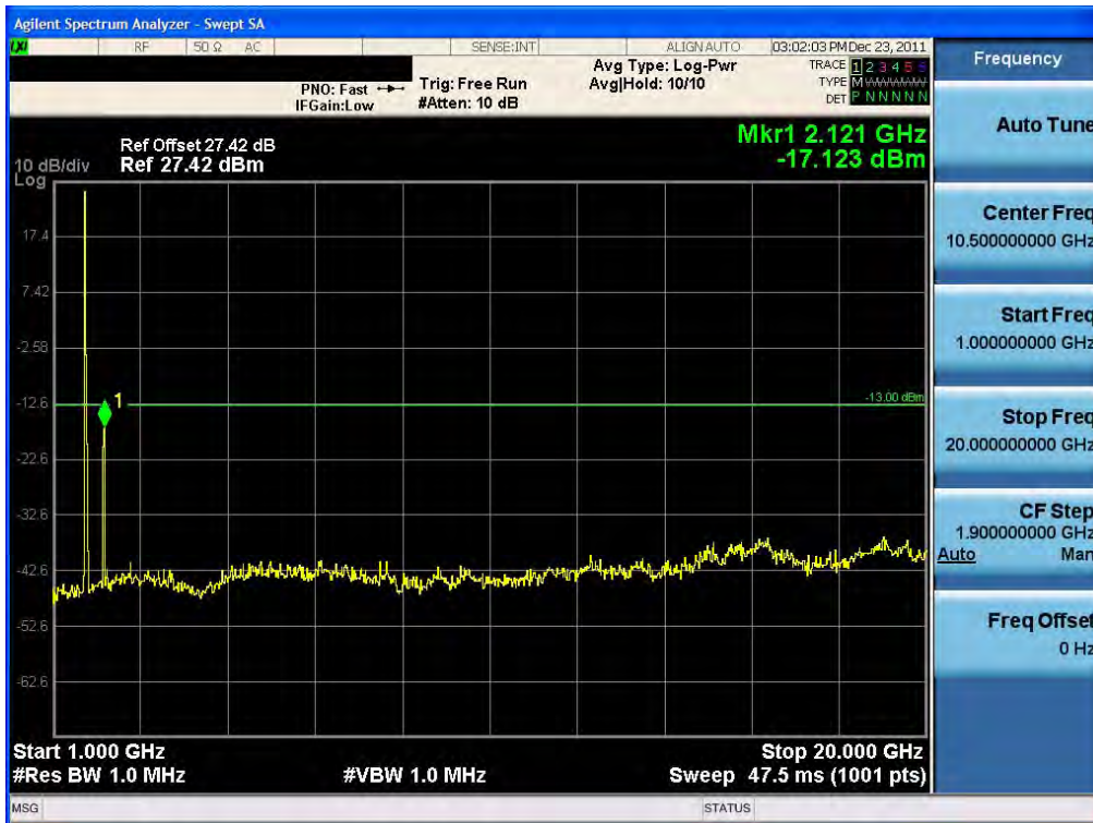
Conducted Spurious Plot (15 MHz BW, 16QAM, Band 4 – Low Channel) RB1-0
