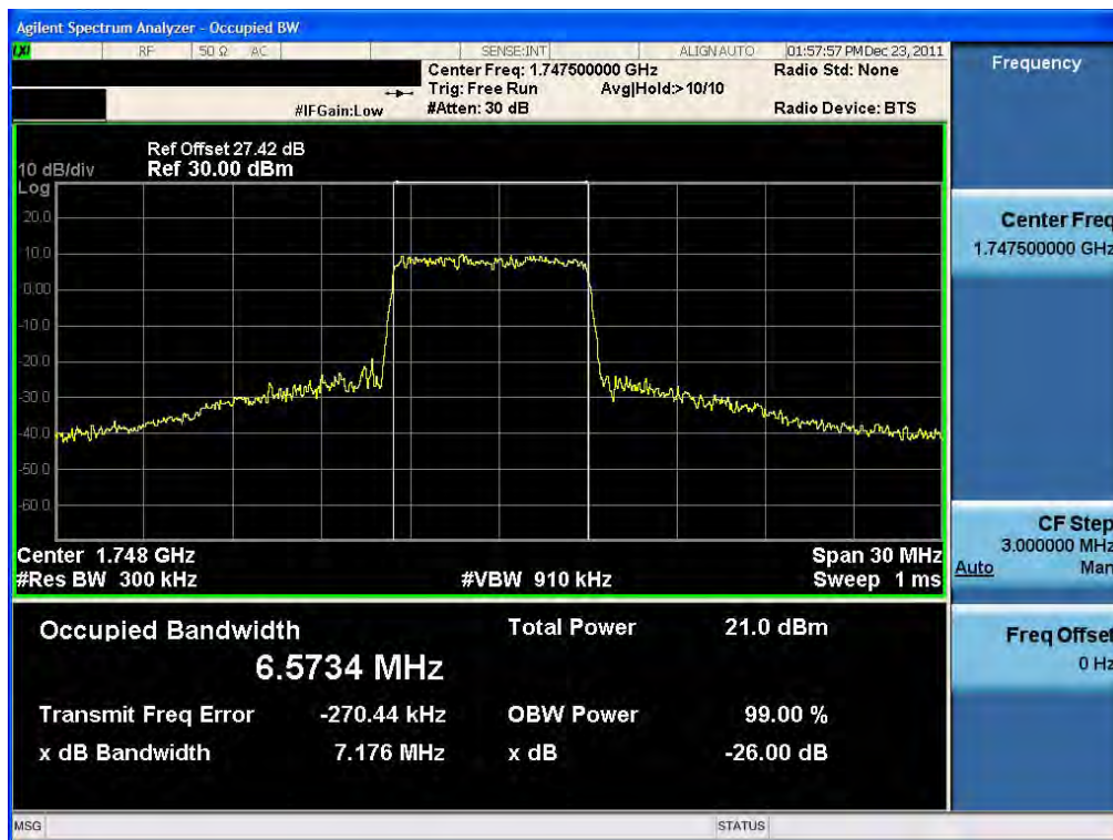
Occupied Bandwidth Plot (15 MHz BW, 16QAM, Band 4 – High Channel) RB36-18
