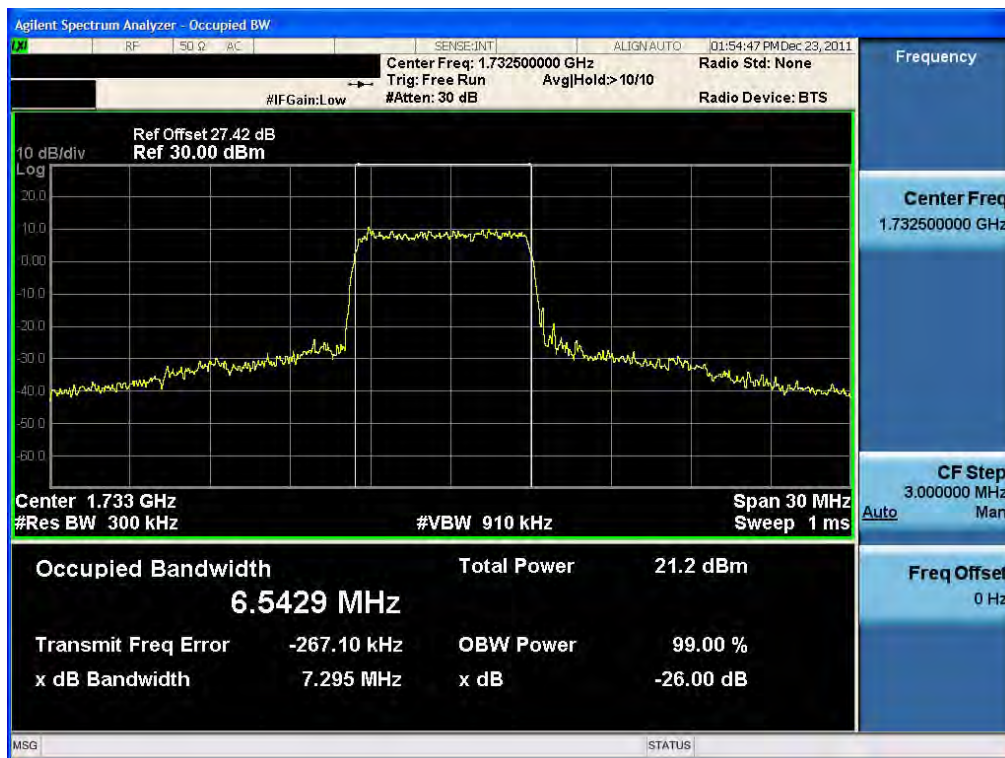
Occupied Bandwidth Plot (15 MHz BW, 16QAM, Band 4 – Mid Channel) RB36-18
