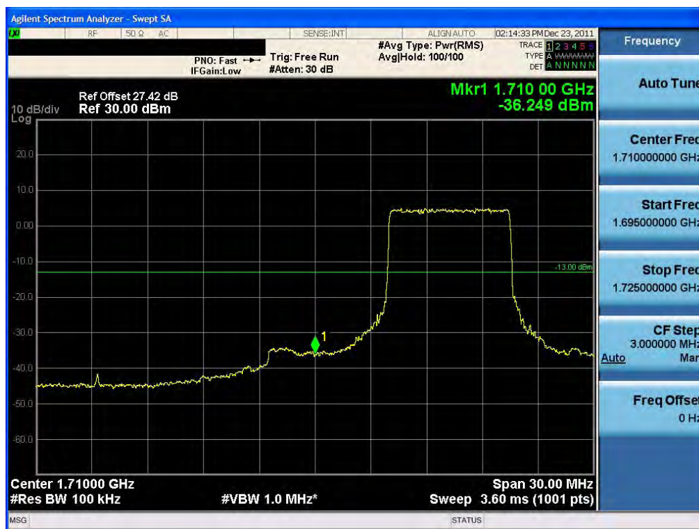
BAND EDGE Plot (15 MHz BW, QPSK, Band 4 – Low Channel) RB36-18
