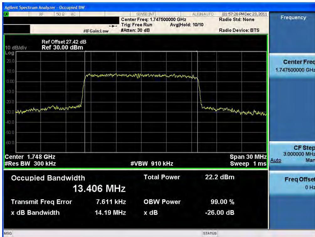
Occupied Bandwidth Plot (15 MHz BW, QPSK, Band 4 – High Channel) RB75-0
