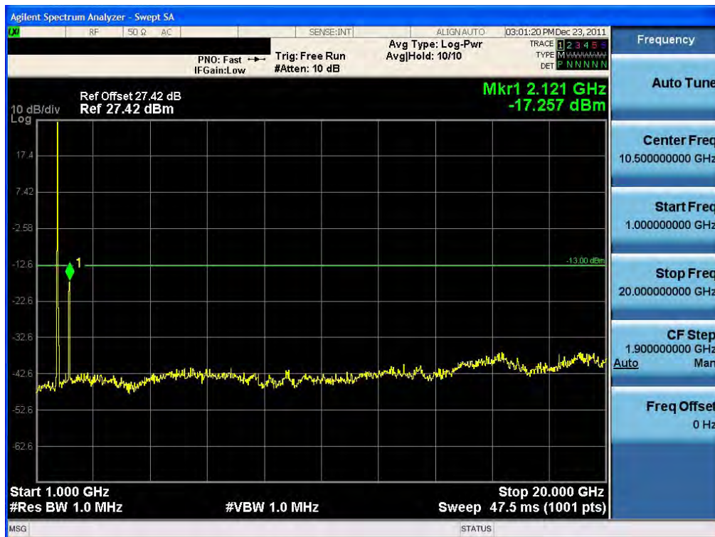
Conducted Spurious Plot (15 MHz BW, QPSK, Band 4 – Low Channel) RB1-74
