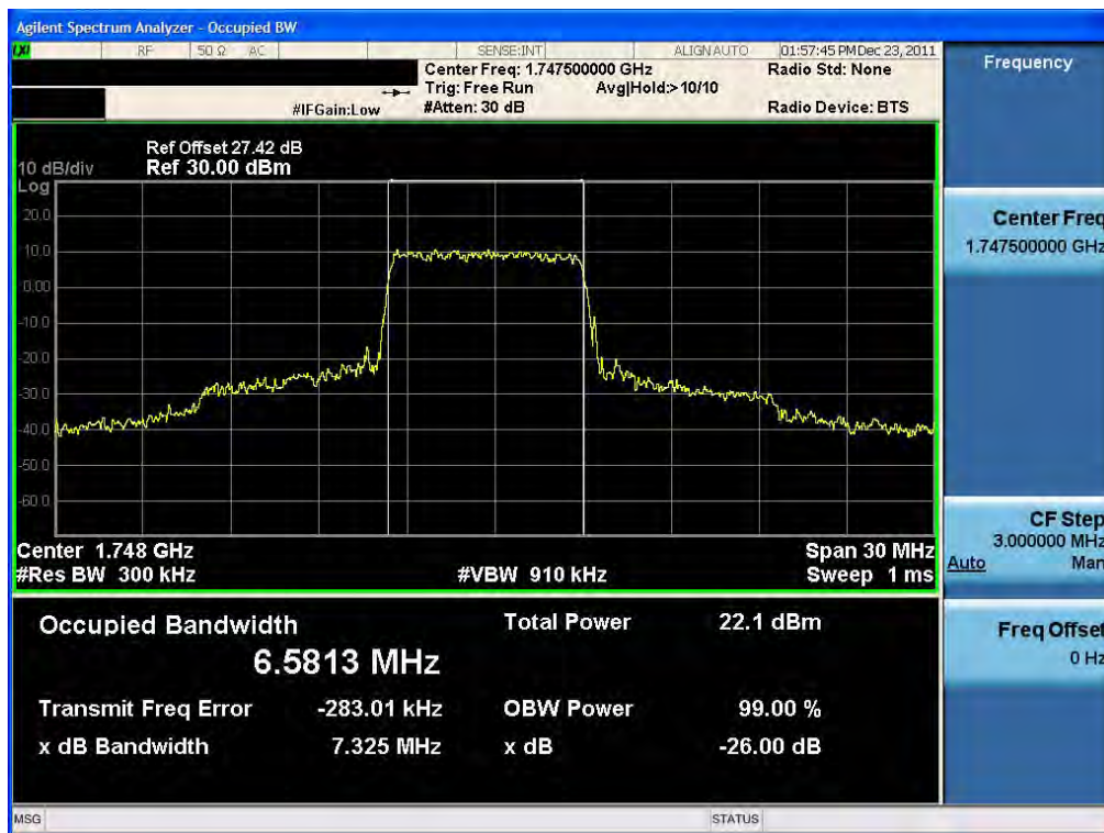
Occupied Bandwidth Plot (15 MHz BW, QPSK, Band 4 – High Channel) RB36-18
