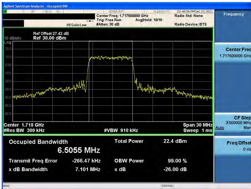
Occupied Bandwidth Plot (15 MHz BW, QPSK, Band 4 -Low Channel) RB36-18
