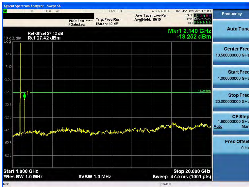
Conducted Spurious Plot (15 MHz BW, QPSK, Band 4 – Mid Channel) RB1-74
