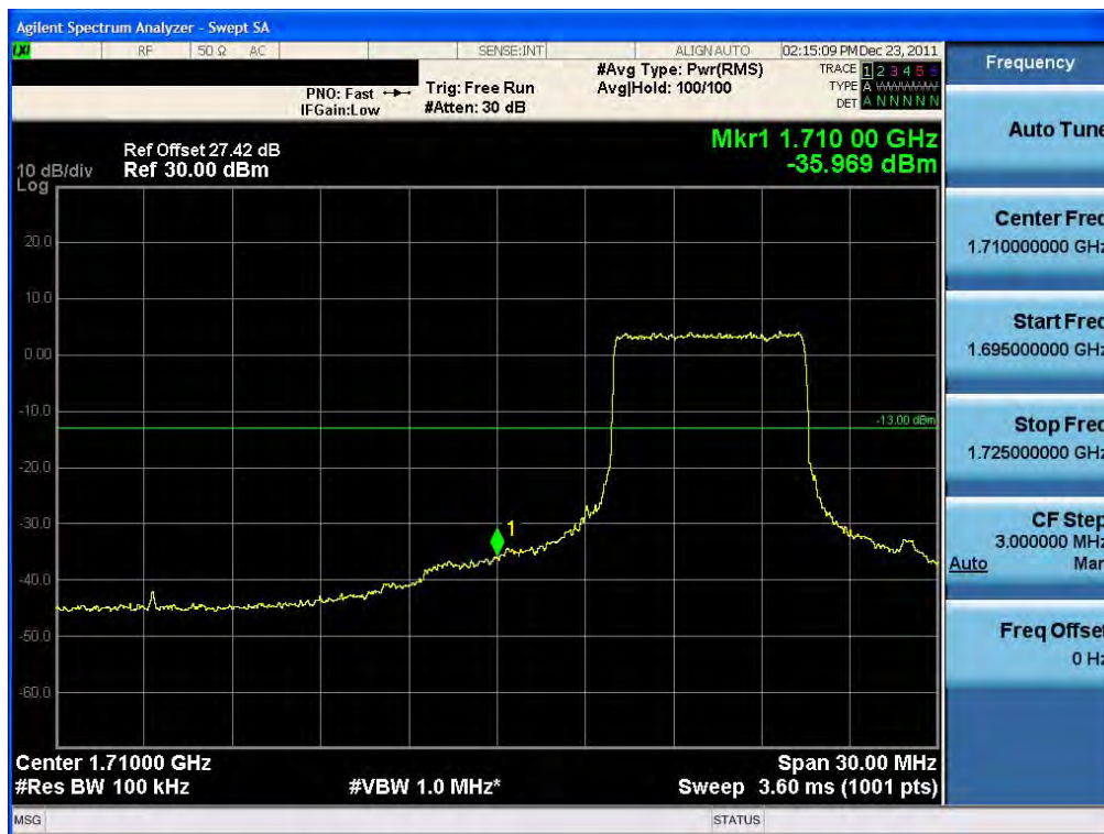
BAND EDGE Plot (15 MHz BW, 16QAM, Band 4 – Low Channel) RB36-18
