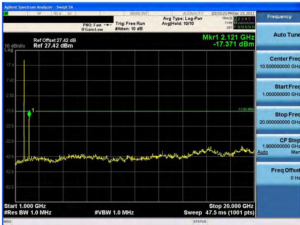
Conducted Spurious Plot (15 MHz BW, QPSK, Band 4 – Low Channel) RB36-18
