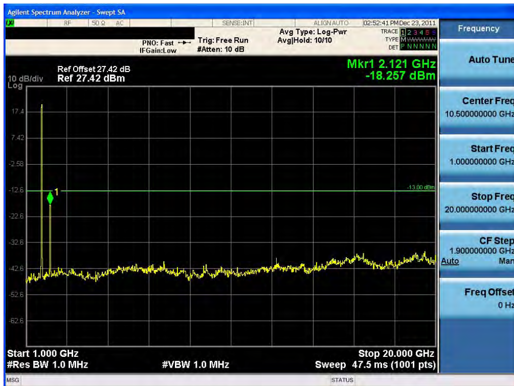
Conducted Spurious Plot (15 MHz BW, 16QAM, Band 4 – Mid Channel) RB36-18
