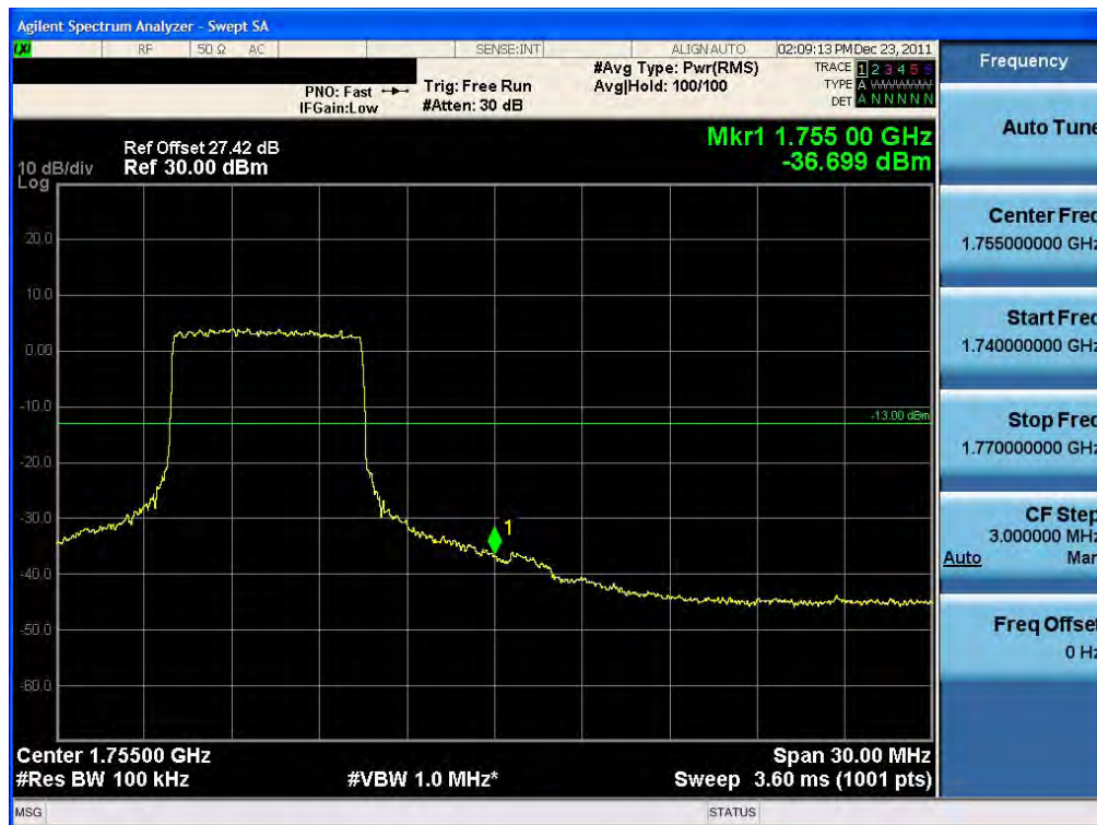
BAND EDGE Plot (15 MHz BW, QPSK, Band 4 – High Channel) RB36-18
