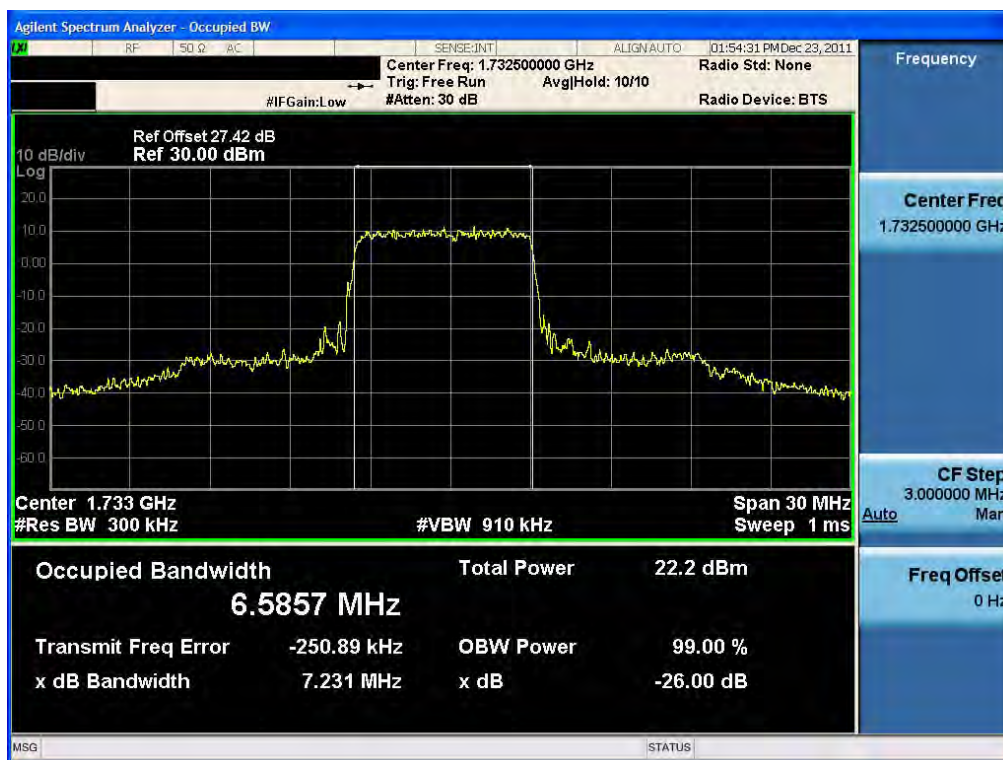
Occupied Bandwidth Plot (15 MHz BW, QPSK, Band 4 –Mid Channel) RB36–18
