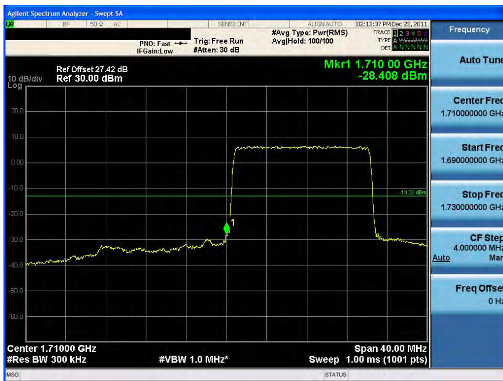
BAND EDGE Plot (15 MHz BW, QPSK, Band 4 – Low Channel) RB75-0
