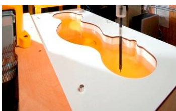
Figure 6-2 SAM Phantom with Simulating Tissue
