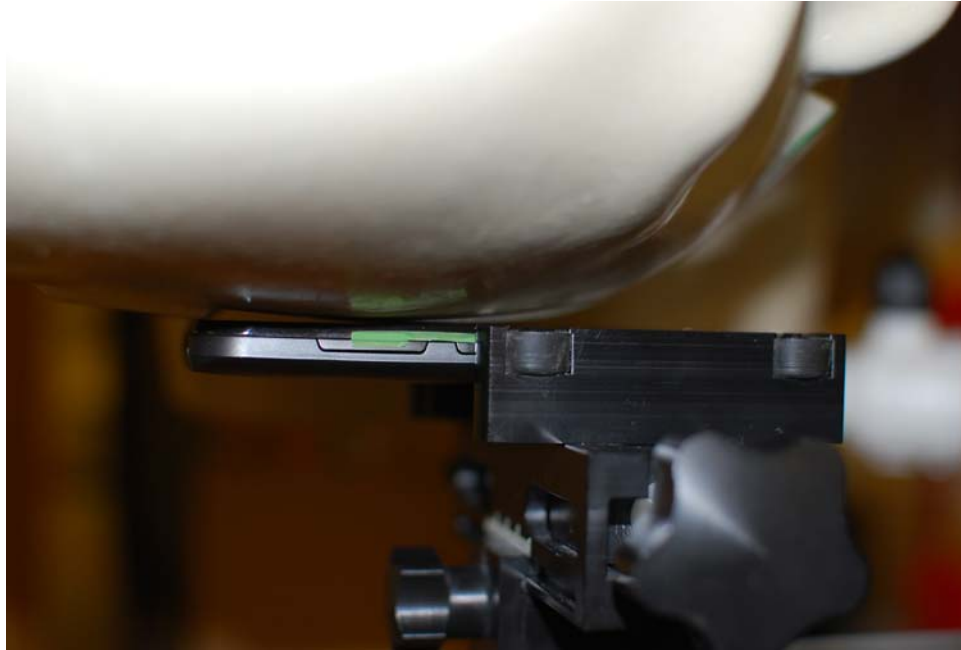
Figure 21-1 SAR Test Setup Photo 1: Right Touch
