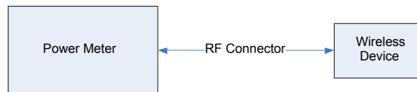
Figure 12-1 Power Measurement Setup
