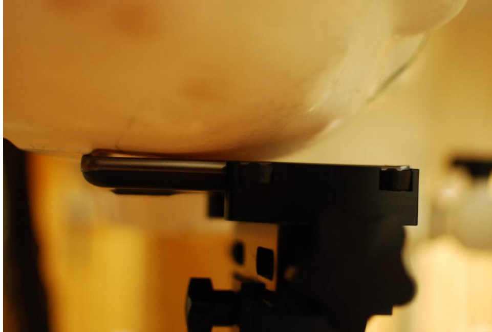
Figure 21-1 SAR Test Setup Photo 1: Right Touch
