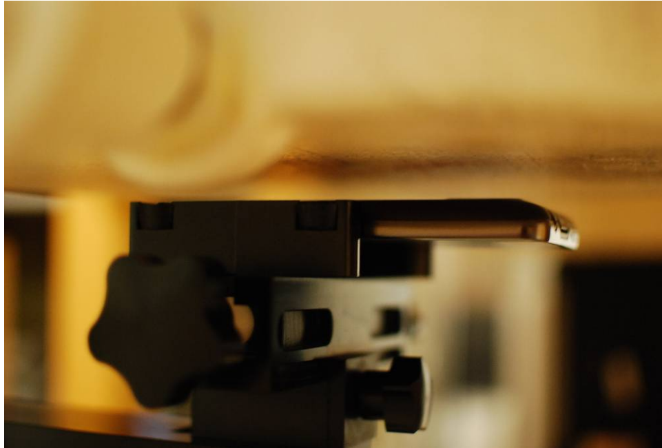
Figure 21-5 SAR Test Setup Photo 5: Back at 1.0 cm
