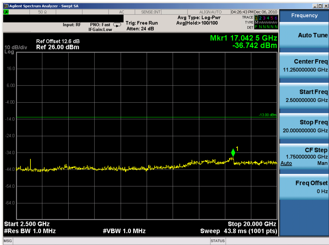
Plot 7-32. Conducted Spurious Plot (AWS WCDMA Mode – Ch. 1862)
