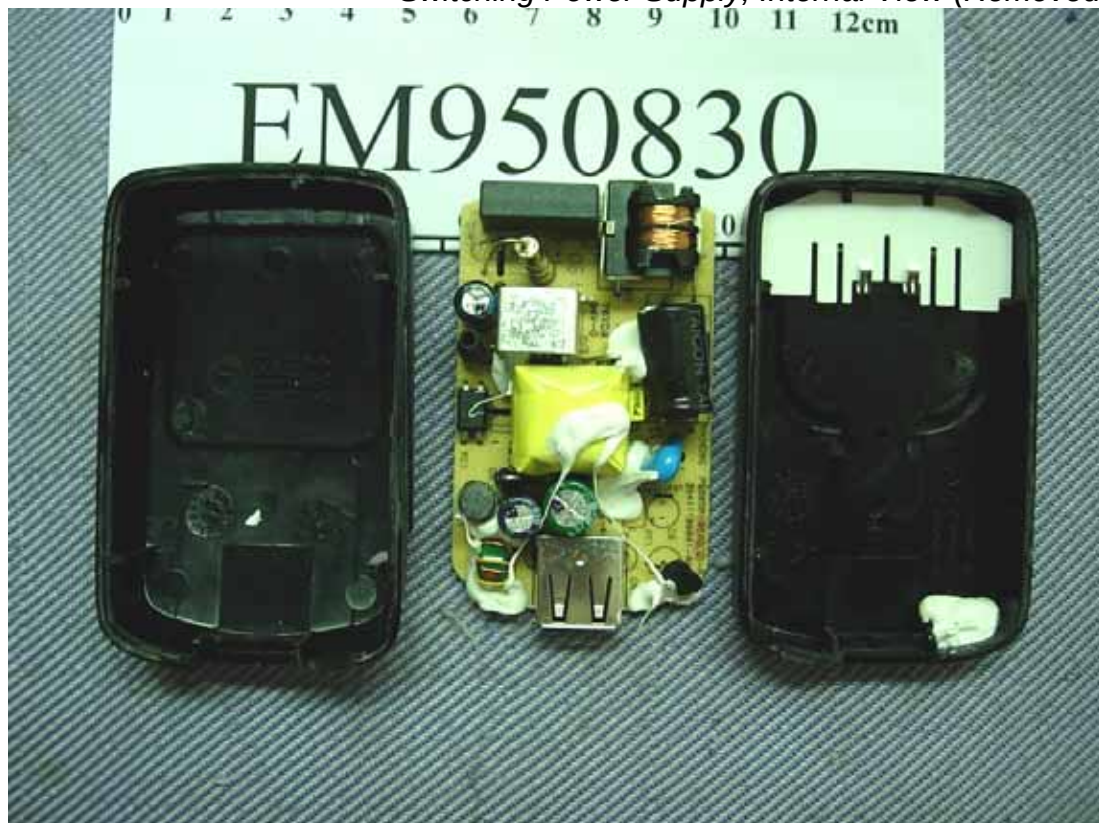
Figure 29 Switching Power Supply, Internal View (Removed Covers)
