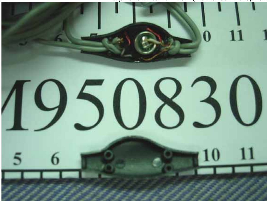
Figure 32 Earphone, Internal View (Removed Microphone Cover)
