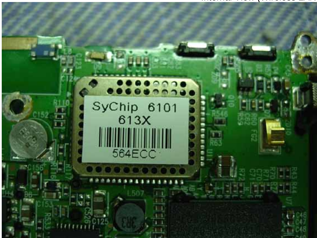
Figure 22 Internal View (Wireless LAN Module)
