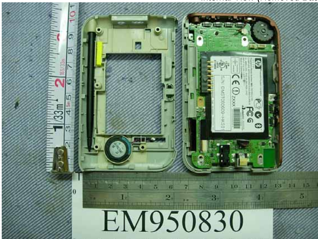
Figure 15 Internal View (Removed Back Cover)
