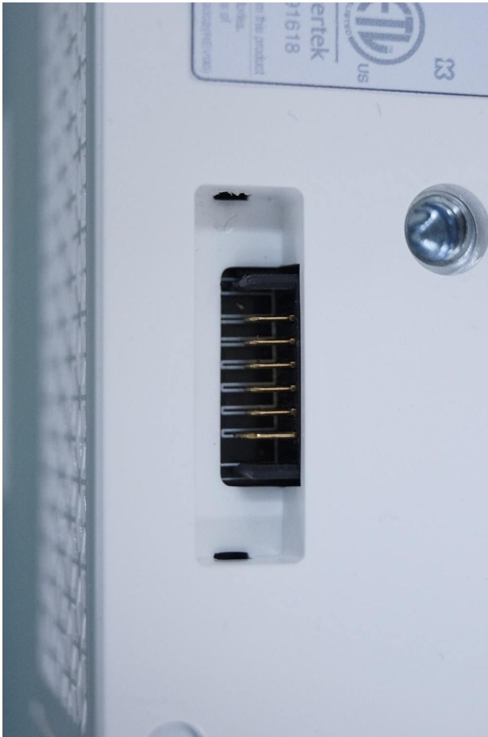
< DC input terminal of Bottom side of EUT >
