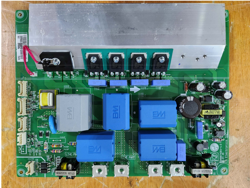
< Inverter 2B PCB (front) >
