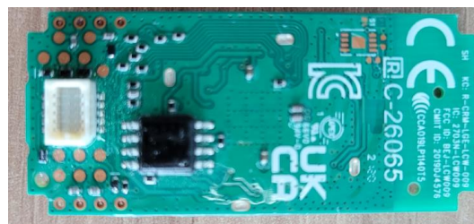
< Wi-Fi module PCB (rear) >
