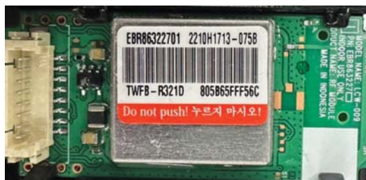
< Wi-Fi module PCB (front) >
