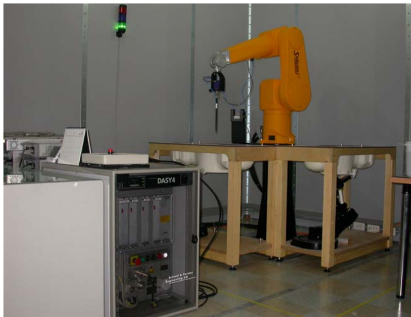
Fig. 4.1 SAR Measurement System
