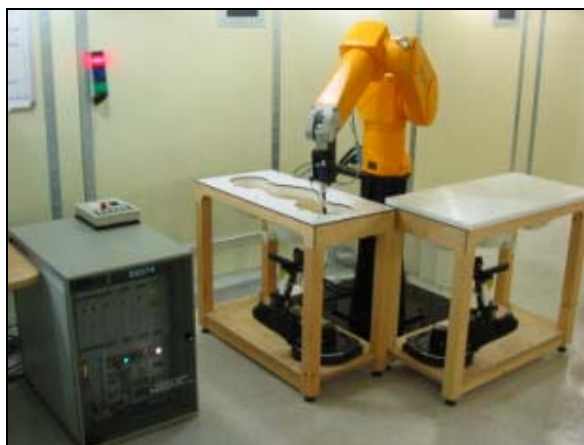
Fig. 4.1 SAR Measurement System
