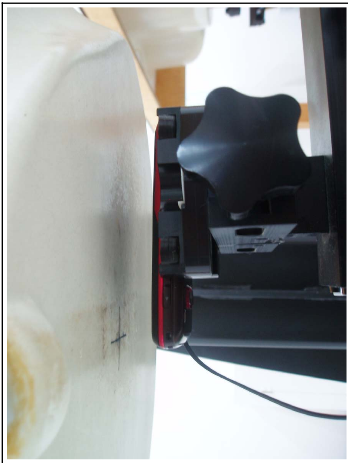
Figure 5 Body SAR Test Setup – w/o Holster
