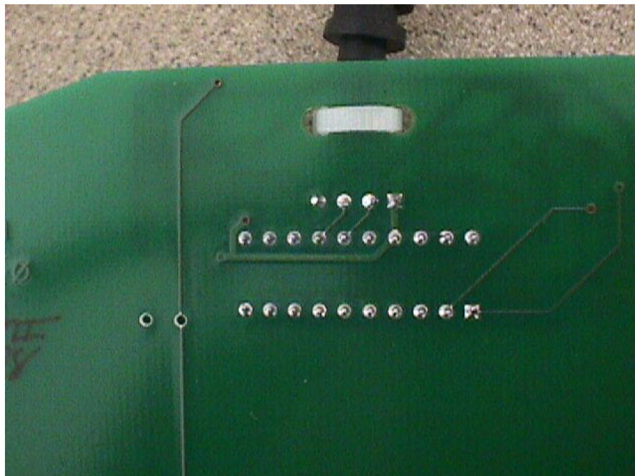
FIGURE 4: Mousepad Solder Side
