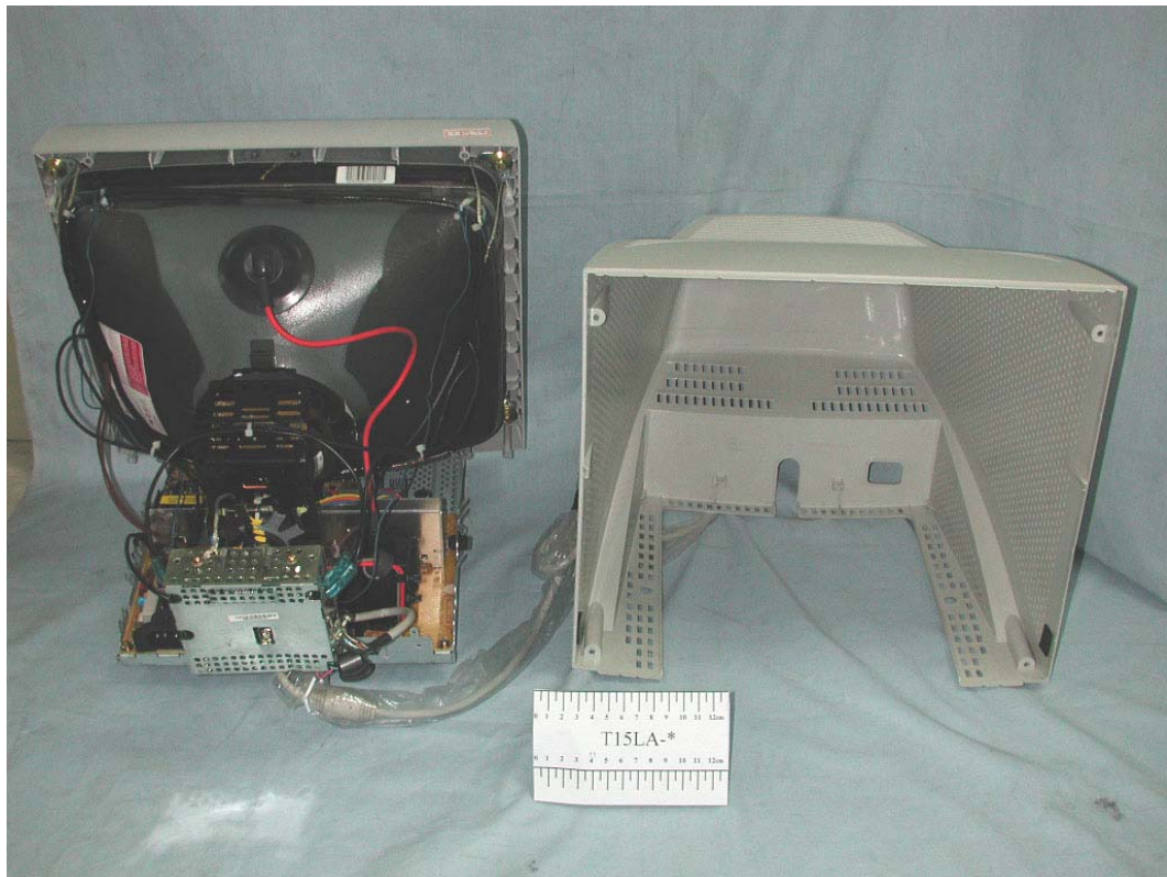
FIGURE 1 COLOR MONITOR (M/N: T15LA-*) COVER REMOVED
