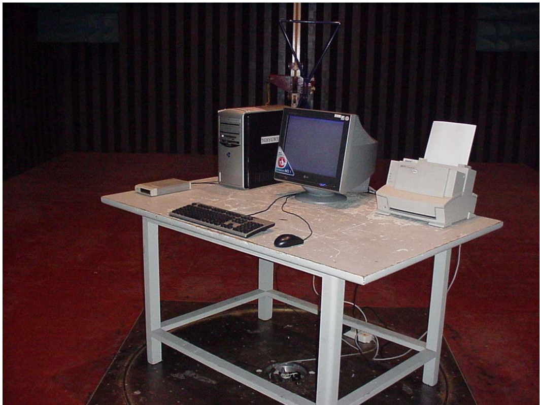
SETUP WITH MAXIMUM DETECTED EMISSION AT VERTICAL POLARIZATION (1024*768@85Hz)
