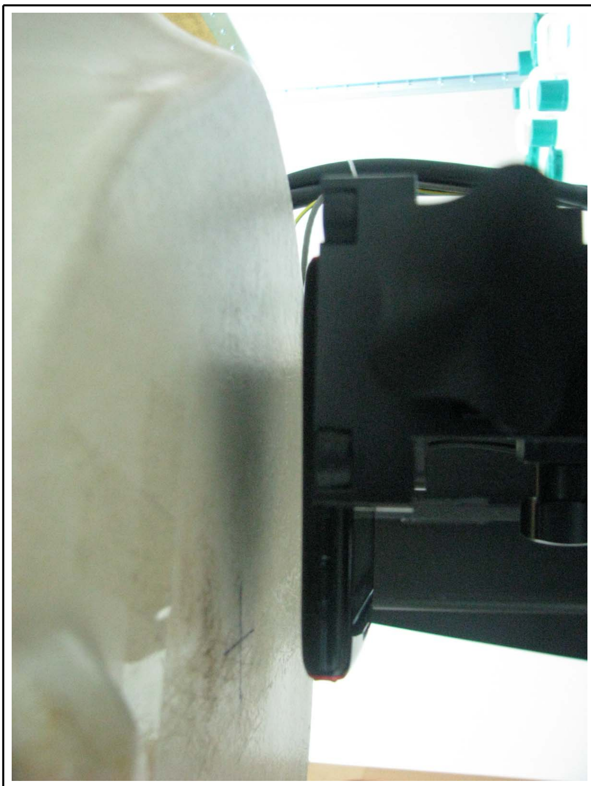
Figure 6 Body SAR Test Setup – w/o Holster
