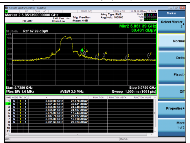
High channel Band edge (Peak) - Band 3
