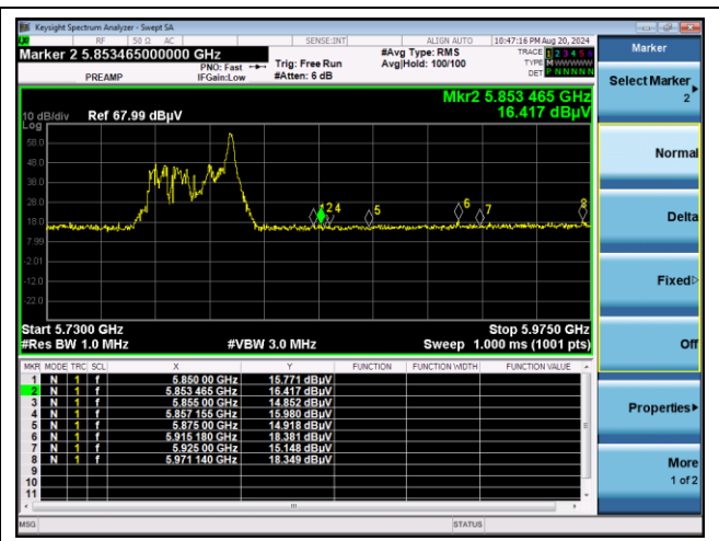
High channel Band edge (Peak) - Band 3
